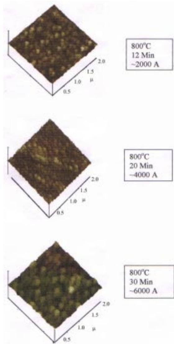
**Figure 1.** AFM images of LCMO films of different thickness for a scan area of  $2 \mu\text{m} \times 2 \mu\text{m}$ . The numbers in the box indicate the substrate temperature, duration of film deposition and the thickness of the grown film.
