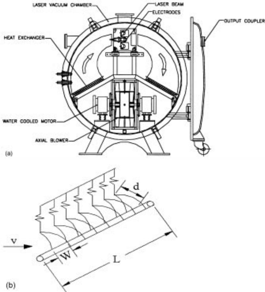
**Figure 1.** (a) Schematic diagram of a transverse flow transversely excited CW CO<sub>2</sub> laser. (b) Schematic diagram of the resistance ballasted multiple pins anode and tubular cathode.
