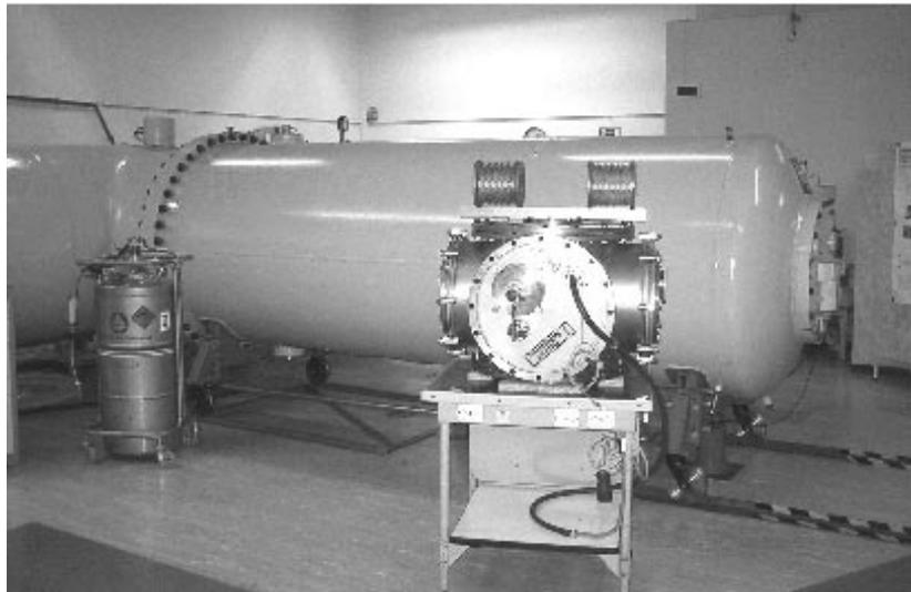
**Figure 4.** Compact  $\text{SF}_6$ -insulated 100 kV tandem accelerator. On the top of the chamber the installed two-acceleration tube modules are shown for comparison. The length of a tube module is 170 mm.
