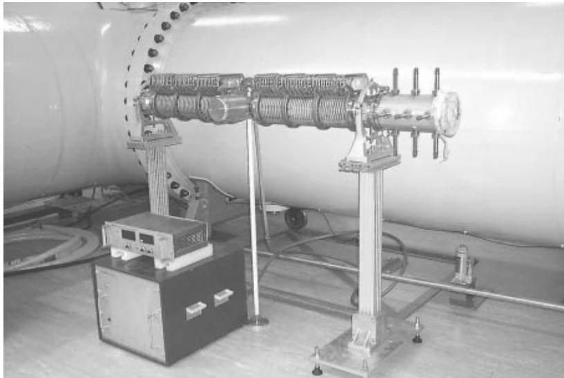
**Figure 1.** Air-insulated 100 kV tandem accelerator in comparison with the 3 MV Tandetron.
