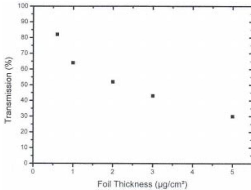
**Figure 3.** Transmission of the AMS facility as a function of the thickness of diamond-like carbon stripper foils.
