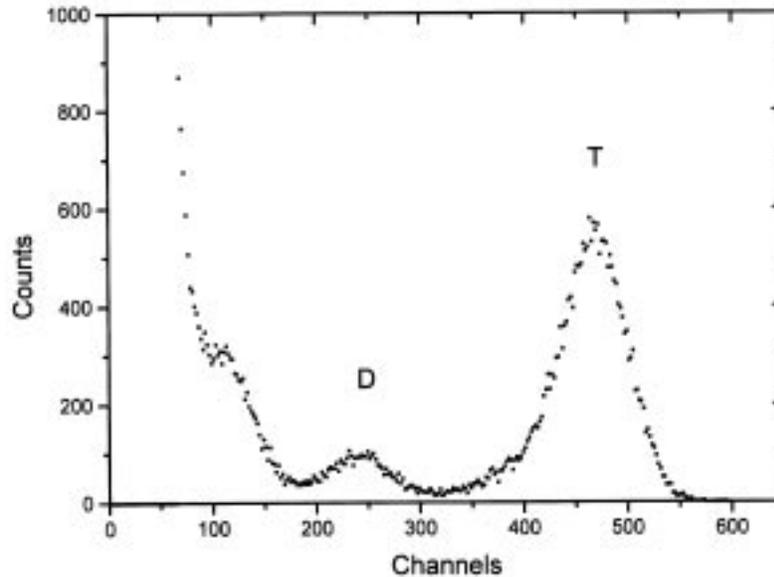
**Figure 2.** Measured energy spectrum of tritium and HD ions.
