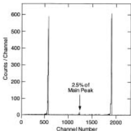
**Figure 8.** Beam time distribution after acceleration without the transmission-line traveling-wave chopper in use. Note both the satellite peak between the two main bunches as well as the improperly accelerated continuum beam tails.
