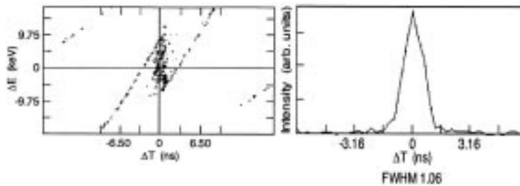
**Figure 3.** Calculated longitudinal phase ellipse created by a first stage four-harmonic buncher. The harmonic buncher is used to form a real time waist upstream of the sine-wave buncher which will then compress this waist by a factor of 4–5 for injection into the PII LINAC.
