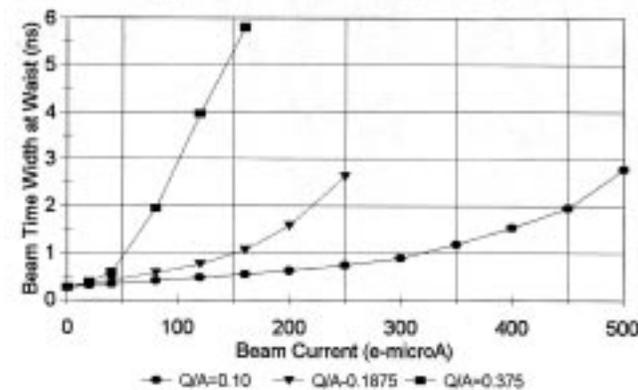
**Figure 5.** Calculated bunch width as a function of total beam current and as a function of ion species charge-to-mass ratio for the new PII bunching geometry. The ability to handle higher beam currents in this system has been improved by at least an order of magnitude.
