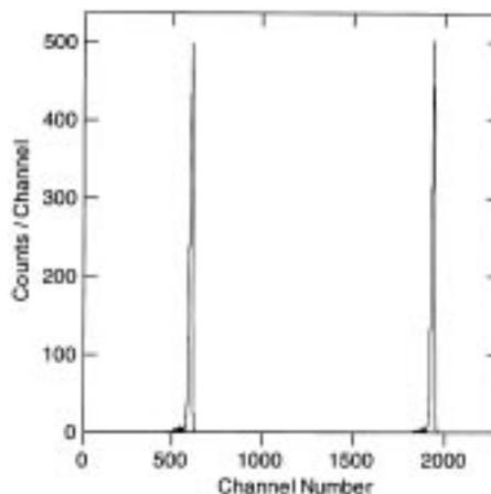
**Figure 9.** Beam time distribution after acceleration with the transmission-line traveling-wave chopper on. The satellite beam peak has been removed as well as the unbunched continuum tails.
