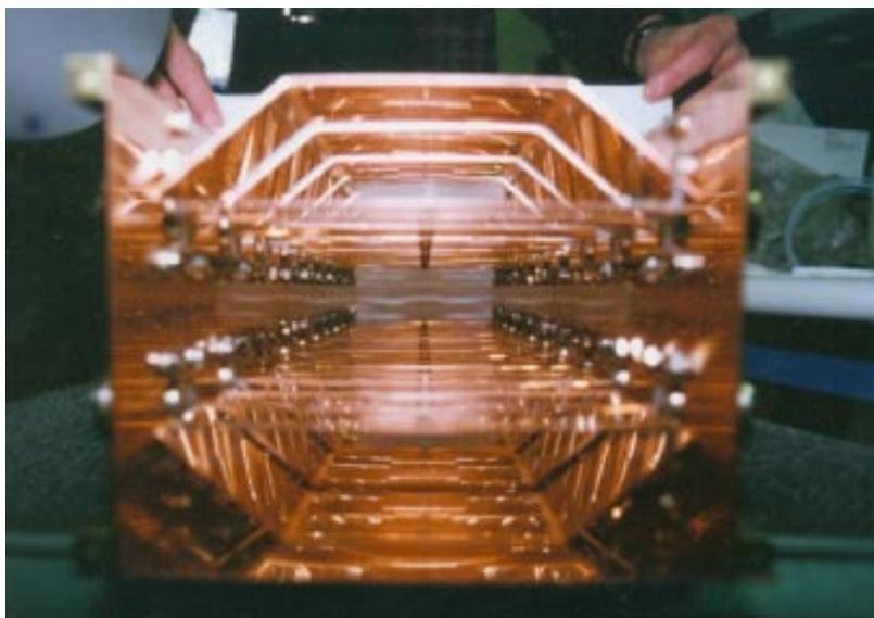
**Figure 6.** Electrode structure of transmission-line traveling-wave chopper.
