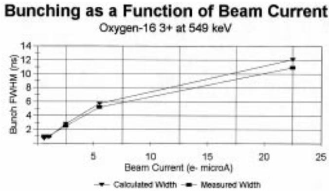
**Figure 2.** Measured beam bunch width achieved with the three-harmonic buncher on the ECR platform for an  $^{16}\text{O}^{3+}$  beam as a function of beam current. The results are compared to the calculated bunch width from a simulation with TRACE-3D [4].
