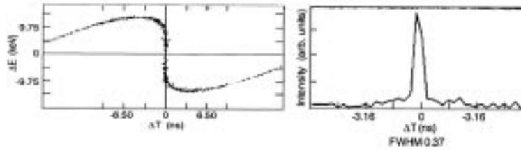
**Figure 4.** Calculated longitudinal phase ellipse created by the combined effects of a first stage four-harmonic buncher and a second stage sine-wave buncher. The harmonic buncher is used to form a virtual time waist downstream of the sine wave buncher. The distortions visible in figure 3 from the imperfect harmonic buncher wave form are not visible in this simulation. The emittance is dominated by the source system energy spread and the distortions are due to the sine-wave buncher.
