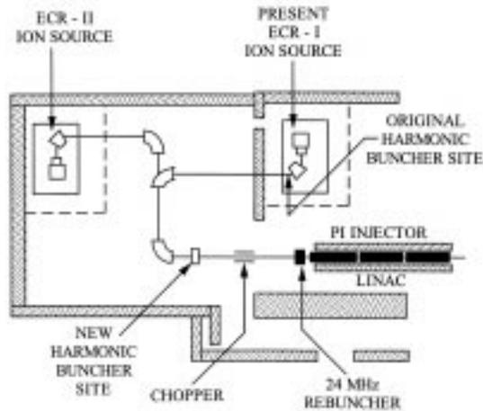
**Figure 1.** Floor plan of the ATLAS positive ion injector showing the relative location of the components of the injector bunching system.
