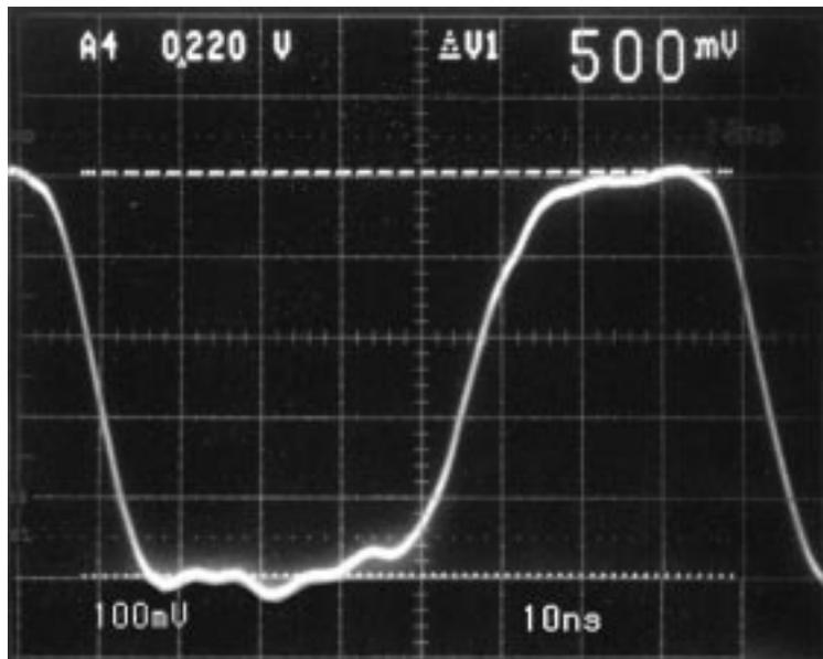
**Figure 7.** Chopper wave form with deflection voltage set for 500 V. The transmission window is 35 ns wide and fall time is approximately 10 ns.
