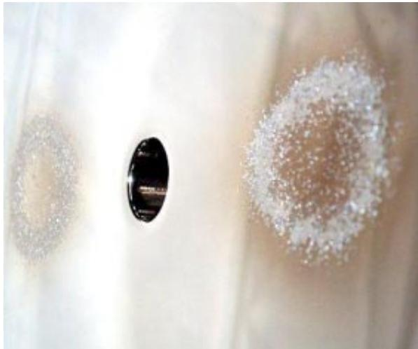
**Figure 7.** High voltage electrode end images on the output plate.
