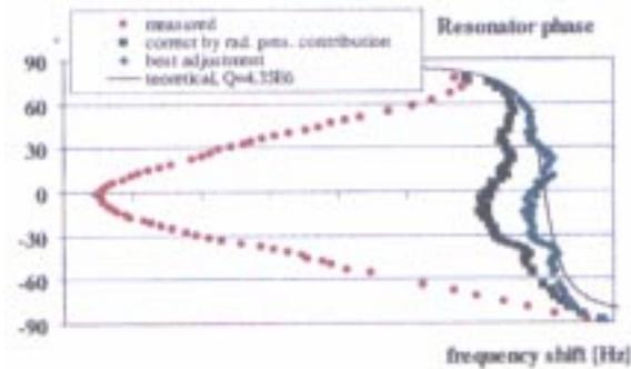
**Figure 11.** Steering of the resonator phase (circles). The curve assumes its theoretical shape (black line) if the measured frequency shifts are corrected by the Lorentz detuning contribution.
