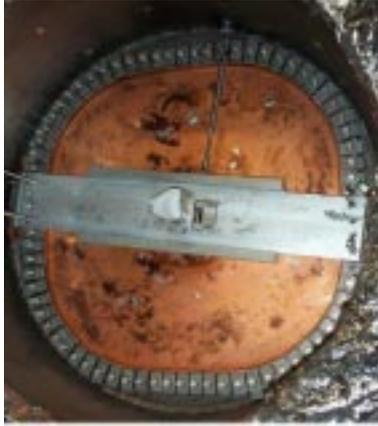
**Figure 4.** The mechanical tuner mounted on its end plate. The pushers, which allow a good electric contact between cavity body and plate without any gasket, are visible on the plate border.
