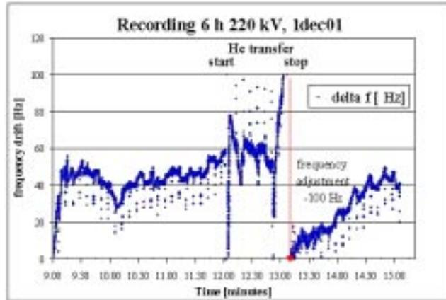
**Figure 12.** Recording of the resonator frequency drifts. At every 730'' spikes are present.
