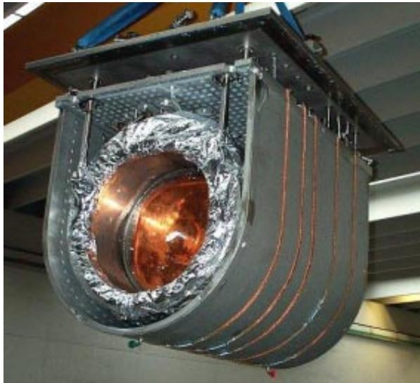
**Figure 3.** SRFQ2 inside the test cryostat during transportation. An end plate of the nitrogen shield was removed for the He tank wrapped in a mylar sheet to be seen. At the center, where the magnetic shield is missing, a resonator end plate is visible.
