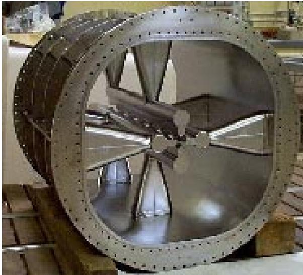
**Figure 1.** SRFQ2 resonator without ending plates before being assembled into the He tank.
