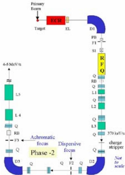
Figure 1. Schematic lay out of the VEC-RIB facility.
