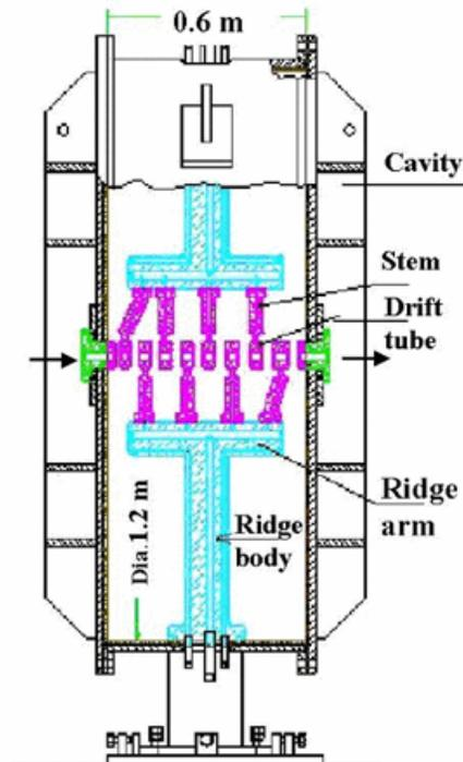
Figure 7. Schematic lay out of the LINAC tank 1.
