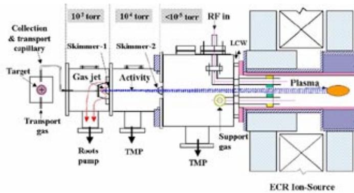
Figure 4. The helium-jet two-stage skimmer assembly.
