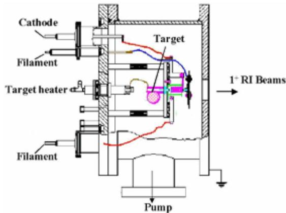
Figure 2. The thick target surface ion source.
