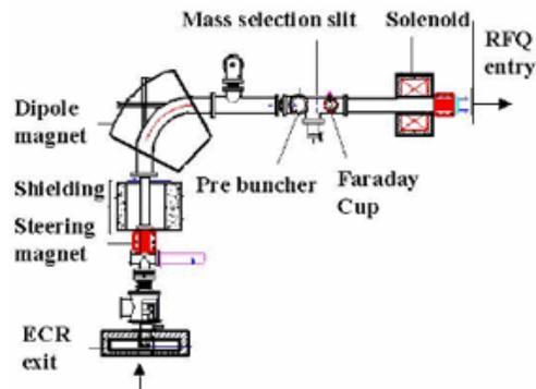
Figure 5. The lay out of ECR to RFQ beam line.
