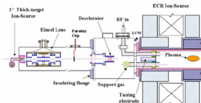
**Figure 3.** The two-ion-source scheme for production of multi-charged RIB.
