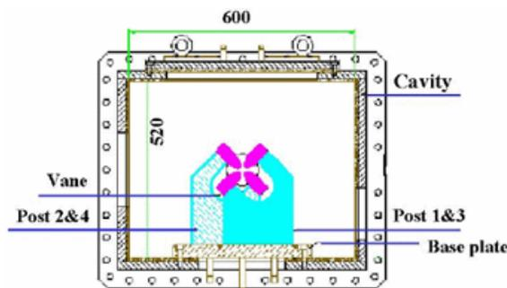
Figure 6. The cross-sectional view of the RFQ cavity.
