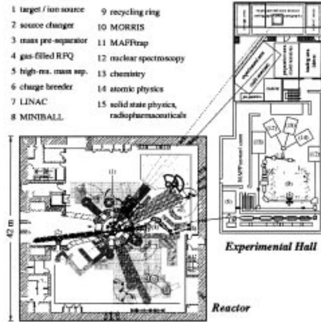
Figure 1. The components of MAFF in the FRM-II building and the external hall.
