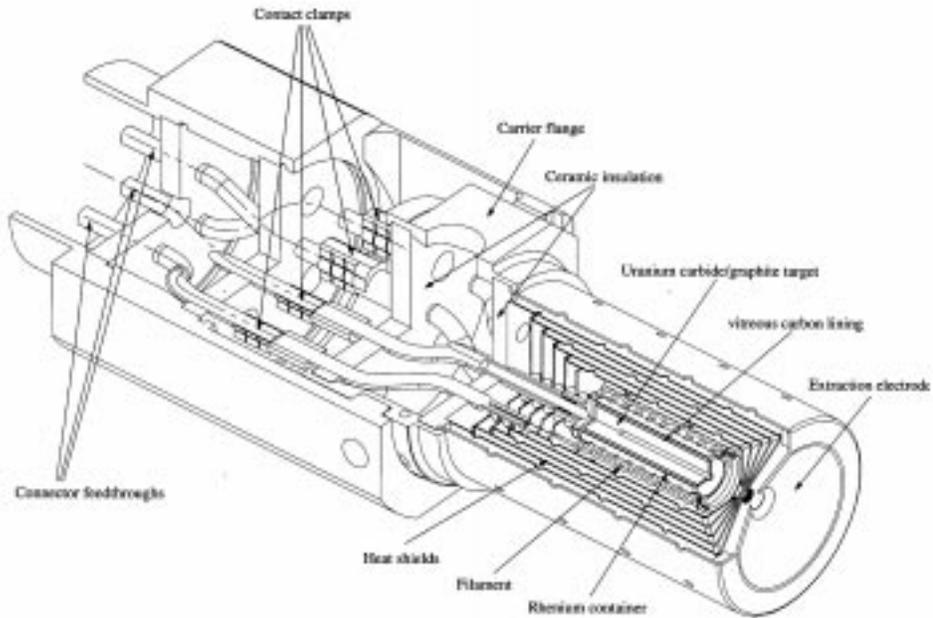
Figure 2. Schematic drawing of the target/ion source unit.
