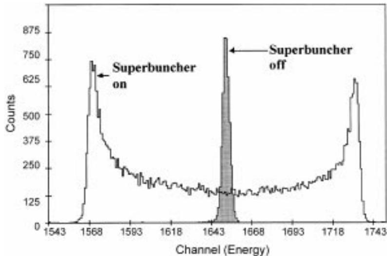
**Figure 1.** The monoenergetic peak with resonator OFF splits into a broad band with two peaks when the resonator is turned ON.
