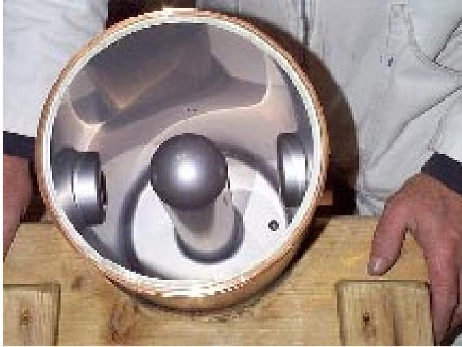
**Figure 1.** A medium  $\beta$  Pb on Cu resonator after being removed from the cryostat.
