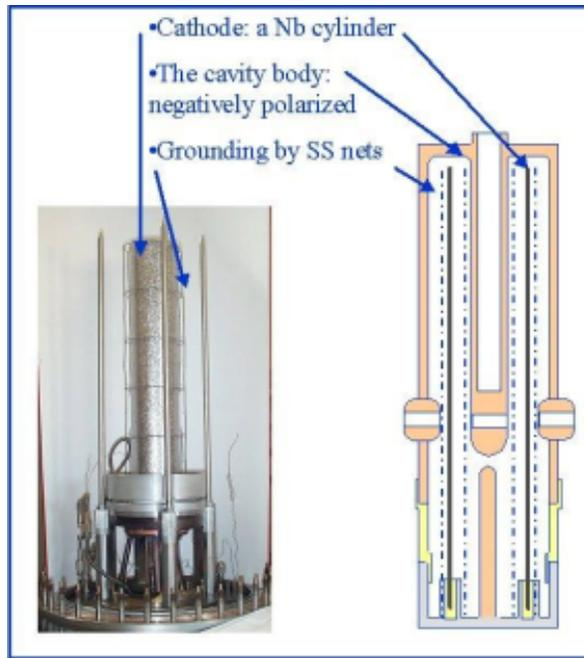
**Figure 4.** The sputtering configuration.
