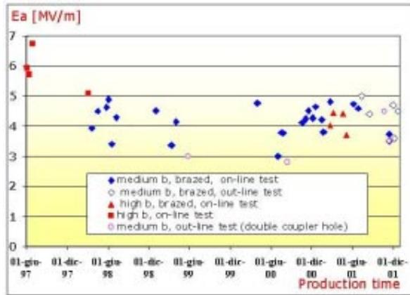
**Figure 6.** Performance as a function of the production time for sputtered medium and high  $\beta$  resonators. Beam energy gain confirmed the calibration of the accelerating field in the installed resonators.
