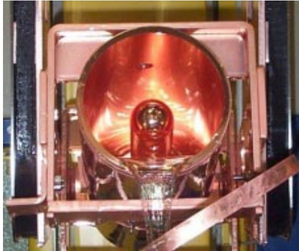
**Figure 3.** The resonator copper base after chemical polishing: the surface is mirror-like.
