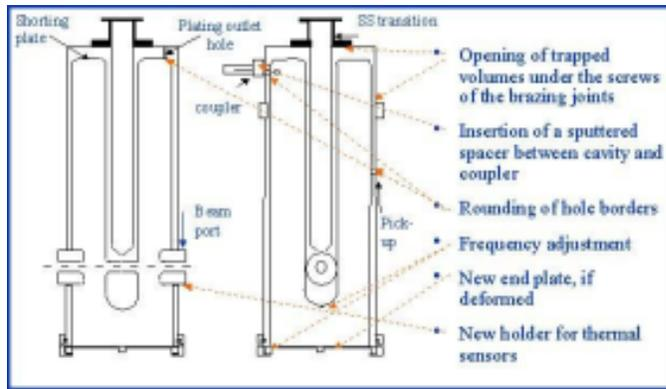
**Figure 2.** Mechanical adjustments of the resonator substrate before the sputtering process.
