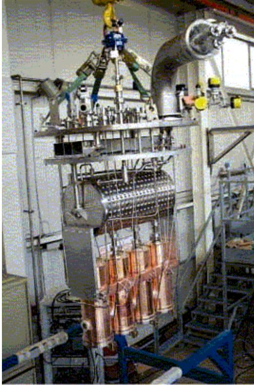
**Figure 5.** The ALPI cryostat completed with four sputtered resonators during the alignment procedure.
