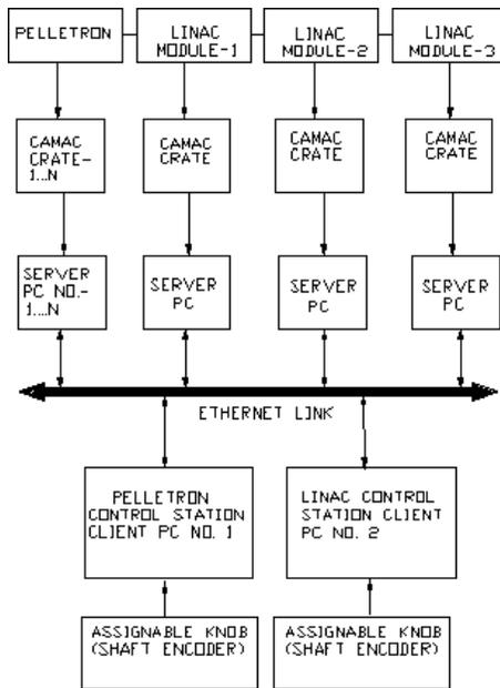
Figure 7. Schematic diagram of the Pelletron-LINAC control system.
