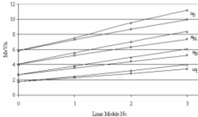
**Figure 2.** Resultant energy per mass unit for different ions from the Pelletron LINAC combination. Triangles are for average accelerating electric field of 4 MV/m and squares are for 3 MV/m in the resonators.
