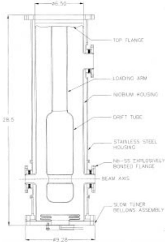
**Figure 3.** Schematic diagram of the quarter wave resonator. Dimensions are in inches.
