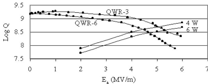
**Figure 4.** Measured values of resonator  $Q$  as a function of accelerating electric field  $E_a$  at 4.5 K.
