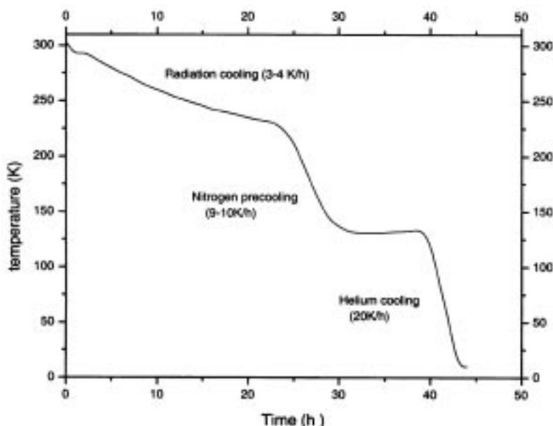
**Figure 5.** Temperature profile of the resonator cool down in the superbuncher cryostat.
