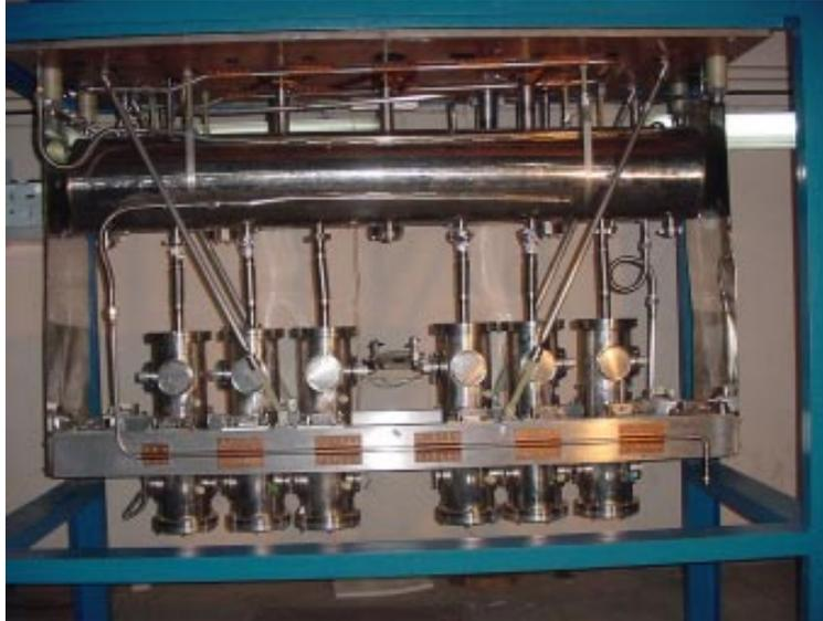
**Figure 6.** Inside view of LINAC cryostat (only six, of the eight, resonators are mounted).
