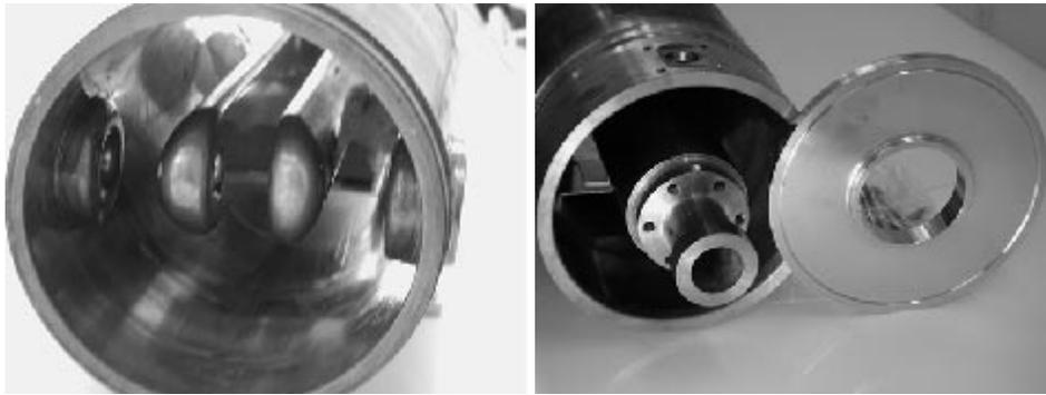
**Figure 3.** Copper prototype for  $\beta = 0.1$ , 150 MHz two-stub resonator using two rf demountable joints between the stub assembly and outer wall. Only one joint will be used in production resonators.
