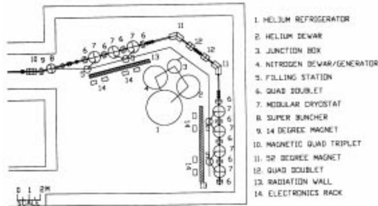
**Figure 2.** A blow up of the various subsystems of the LINAC. The cryogenic plant and the distribution system are also seen in this figure.
