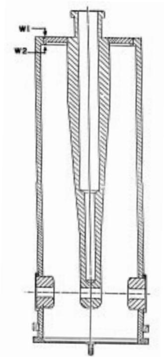
**Figure 3.** The 150 MHz quarter wave resonator.
