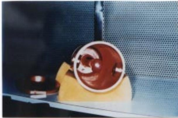
**Figure 4.** Photograph of an indigenously fabricated QWR and its end plate.
