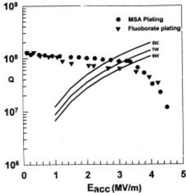
**Figure 5.** The quality factor  $Q$  plotted as a function of the accelerating field in the cavity for lead films prepared using different electrochemical baths.
