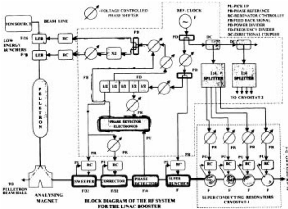
Figure 8. Schematic view of the Pelletron–LINAC beam stabilization scheme.
