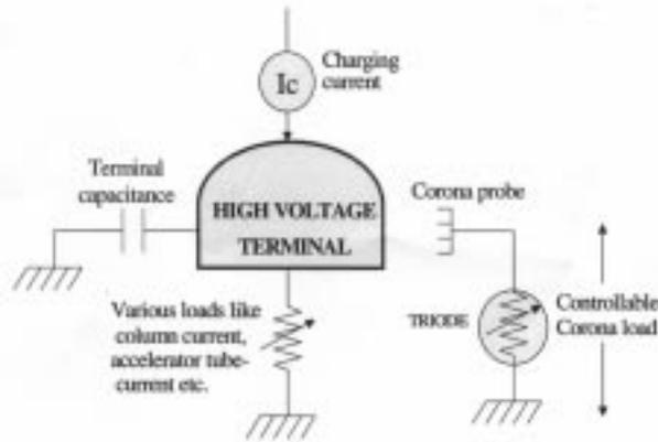
Figure 2. Schematic load distribution.
