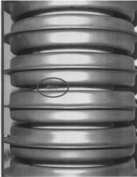
**Figure 6.** Crack in column support post.
