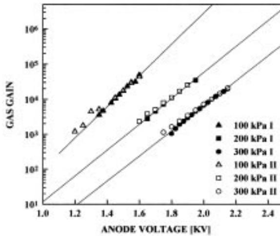
**Figure 6.** Gas gain as a function of anode voltage for various P-10 gas pressures. Two sets of data are shown for each pressure.
