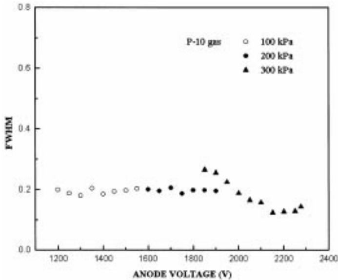
**Figure 5.** Resolution (FWHM) of the main peak as a function of anode voltage for different gas pressures.
