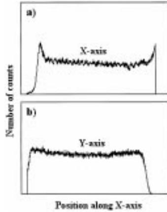
**Figure 9.** Uniform irradiation response of the detector. (a) The upper X-cathode response and (b) lower Y-cathode response.
