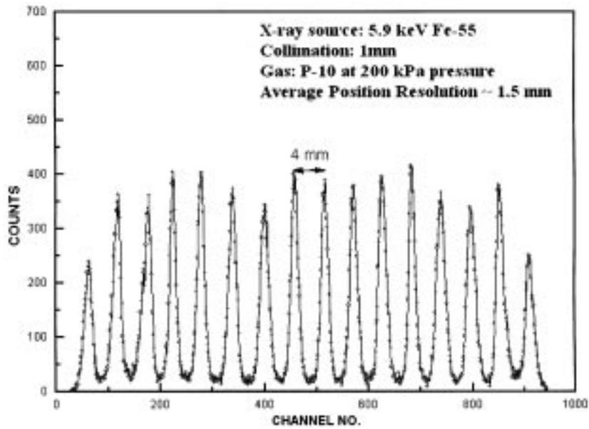
Figure 7. Position response of the detector along X-direction.
