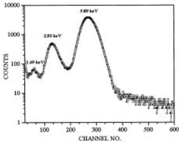
**Figure 4.** Pulse height spectrum of figure 3 in a logarithmic scale, showing the three distinct X-ray energy peaks.
