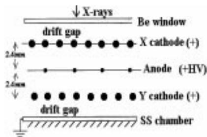
Figure 1. Schematic drawing of the 2-D PSD.
