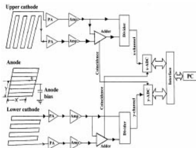
**Figure 2.** Charge division method for position encoding in 2-D PSD.
