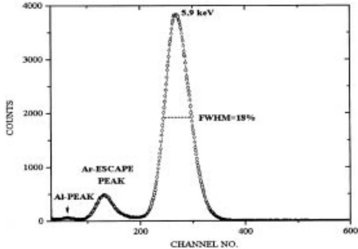
**Figure 3.** Pulse height spectrum for  $^{55}\text{Fe}$  X-rays with P-10 gas at 100 kPa and anode voltage of 1500 V.
