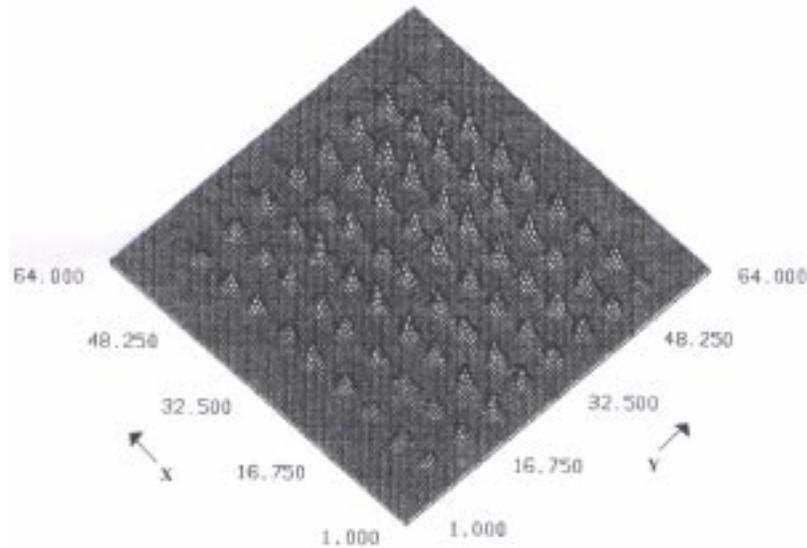
**Figure 10.** Position spectrum obtained with detector covered with a grid containing uniform holes and flooded with X-rays.
