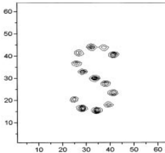
Figure 8. Position spectrum of the character 'S' traced by keeping the X-ray source on various positions of the active area.
