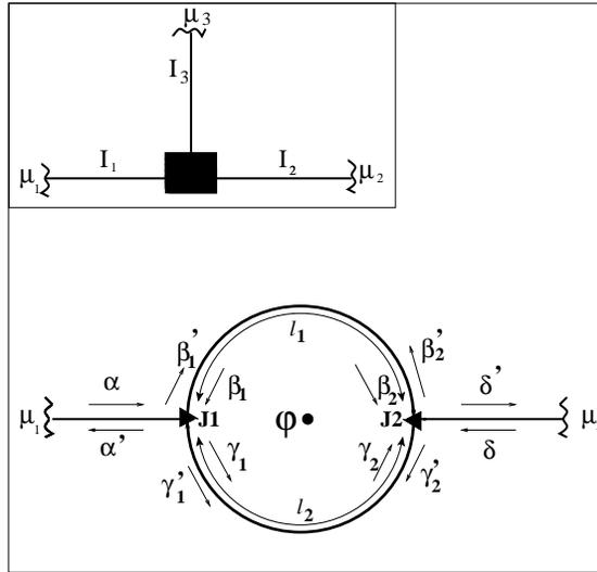
**Figure 1.** Aharonov–Bohm ring geometry. Inset shows the three-probe model.
