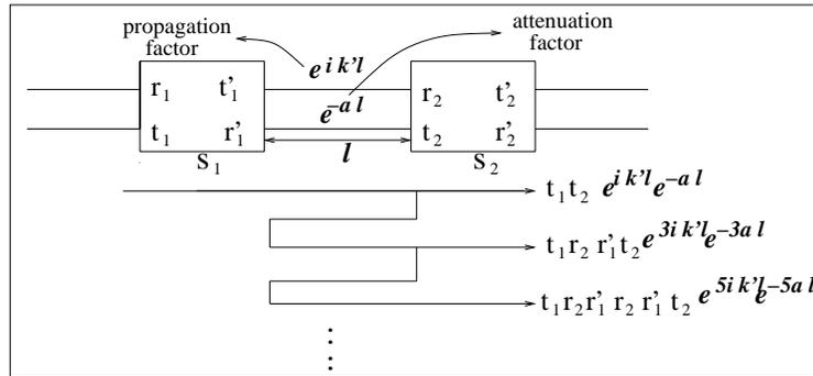
**Figure 4.** Summing the different paths,  $S_1$  and  $S_2$  denote the two scatterers.  $l$  is the distance between them.  $e^{ik'l}$  and  $e^{-\alpha l}$  denote the propagation and attenuation factors in the locality of interest.
