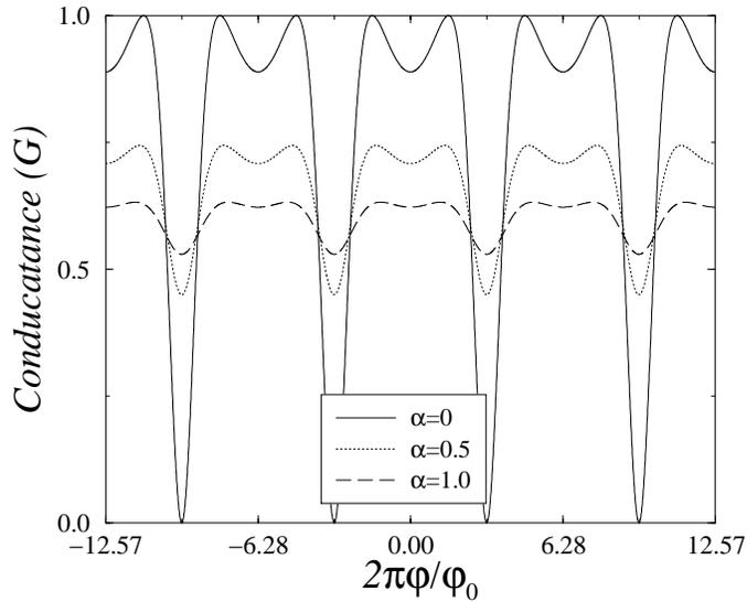
**Figure 2.** Reduction of Aharonov–Bohm oscillations in the presence of incoherence parameter  $\alpha$ .  $kl = \pi$ ,  $l_1/L = 0.75$ ,  $l_2/L = 0.25$ , and coupling  $\varepsilon = 0.5$ .
