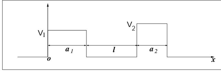
**Figure 5.** The double heterostructure. Barriers are denoted by their width  $a_j$  and height  $V_j$ ,  $j = 1, 2$ . The width of the well is  $l$ .
