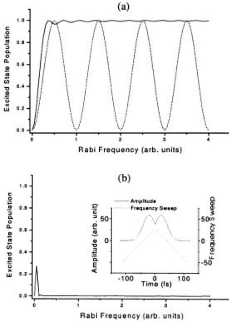
**Figure 4.** (a) Relative excited state population for 2-photon excitation (overlapped Gaussian envelop) as a function of Rabi frequency for a transform-limited (dashed line) vs. a bandwidth equivalent frequency-swept (solid line) pulse. (b) However, when the frequency sweep of the second pulse in the two-photon excitation is reversed with respect to the first pulse (see inset), a counter-intuitive self-induced transparency occurs.
