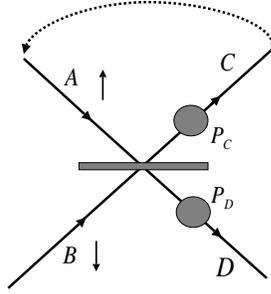
**Figure 1.** The set-up for generating entangled states using quantum indistinguishability. The feedback loop is shown in the figure as a dotted line. If the particles bunch in the same output channel, they are fed back into the beamsplitter. This is recursively continued till the particles anti-bunch, in which case they are entangled.
