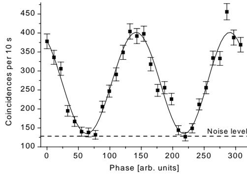
**Figure 3.** Two-photon interference fringes. According to a sinusoidal fit, the visibility is  $97\pm 5\%$  after subtraction of the accidental coincidences.
