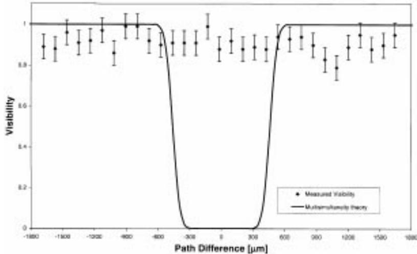
**Figure 4.** Visibility vs. path difference, the plain curve corresponds to the predictions of multisimultaneity theory
