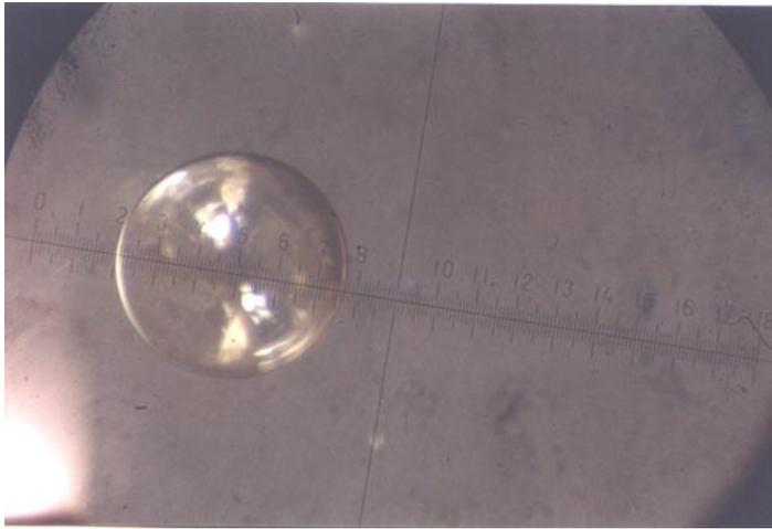
**Figure 8.** Optical micrograph of a polystyrene microsphere, diameter 1452  $\mu\text{m}$ .
