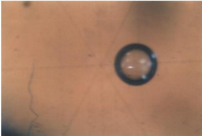
**Figure 9.** Optical micrograph of a thick-walled polystyrene microsphere, diameter 863  $\mu\text{m}$ .
