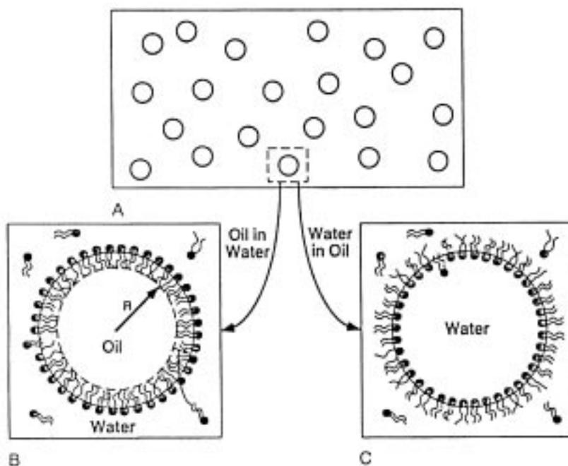
**Figure 2.** (A) Droplet emulsion phase, (B) oil-in-water (O/W), (C) water-in-oil (W/O) type.
