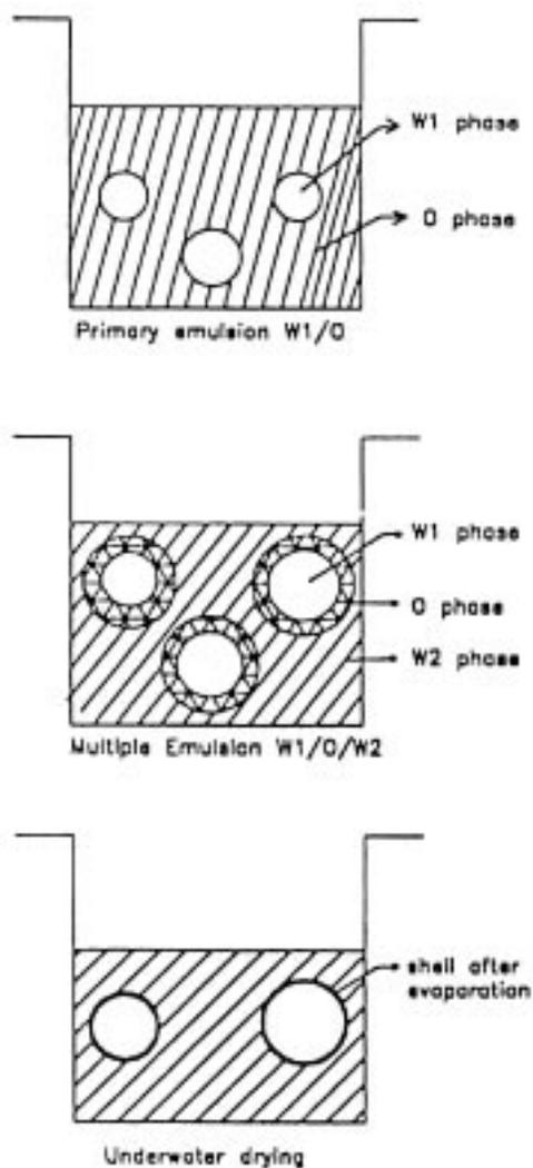
**Figure 6.** Schematic diagram of density-matched emulsion technique.
