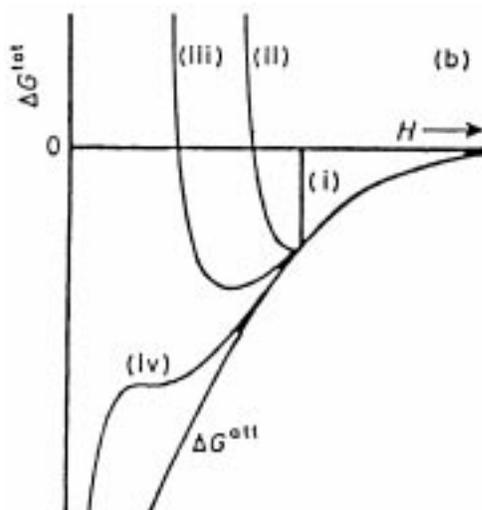
**Figure 5.** Total interaction free energy curves for sterically stabilized colloidal systems.
