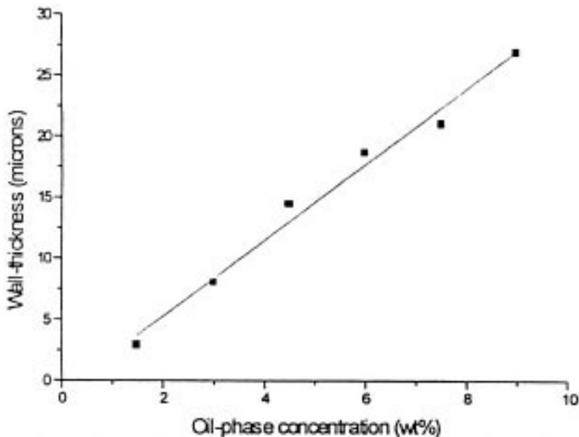
**Figure 7.** Relationship between wall thickness of the microsphere and oil-phase concentration.
