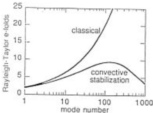
**Figure 1.** Typical number of exponentiations of the ablative Rayleigh–Taylor instability during an implosion. The upper classical curve assumes a growth rate proportional to square root of  $ka$ . The lower curve includes ablative (convective) stabilization. The maximum growth is near 100.
