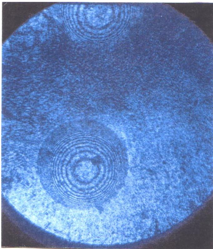
**Figure 10.** An interferogram of a microsphere showing circular fringe pattern.
