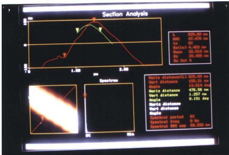
Figure 14. Measurement of wall thickness of PS layer of a microsphere.
