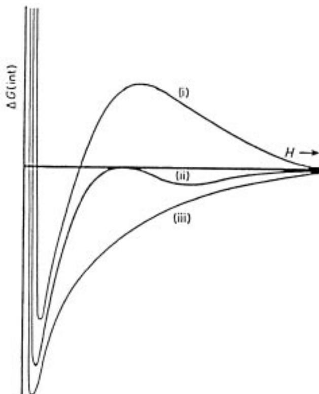
**Figure 4.** Total interaction free energy for electrostatically stabilized colloidal system.
