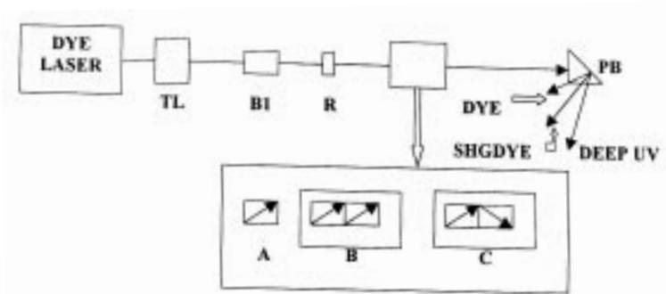
**Figure 2.** The schematic illustration of the experimental arrangements for THG. TL – The telescopic arrangement, B1 – Type-I,  $\theta = 30^\circ$  cut, 7.3 mm thick crystal, R –  $90^\circ$  polarization rotator for the second harmonic of dye laser radiation. A, B and C are three different configurations for THG, A – Single crystal, B – two crystals (B2 and B3 in NWOC), C – two crystals (B2 and B3 in WOC) with the optic axes directions as shown in the figure. PB – Pelin Broca prism.
