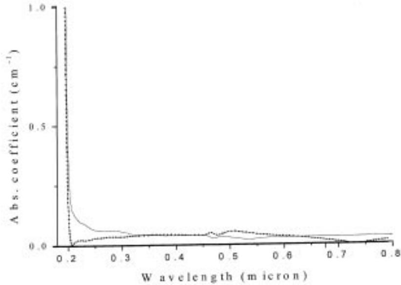
**Figure 1.** The optical transmission characteristics of BBO crystals at room temperature. Solid curve – Type-I,  $\theta = 30^\circ$  cut, 7.3 mm thick crystal, grown at NEC, Japan. Dotted curve – Type-I,  $\theta = 67^\circ$  cut, 12 mm thick crystal, grown at Institute of Mineralogy and Petrography, Russia.
