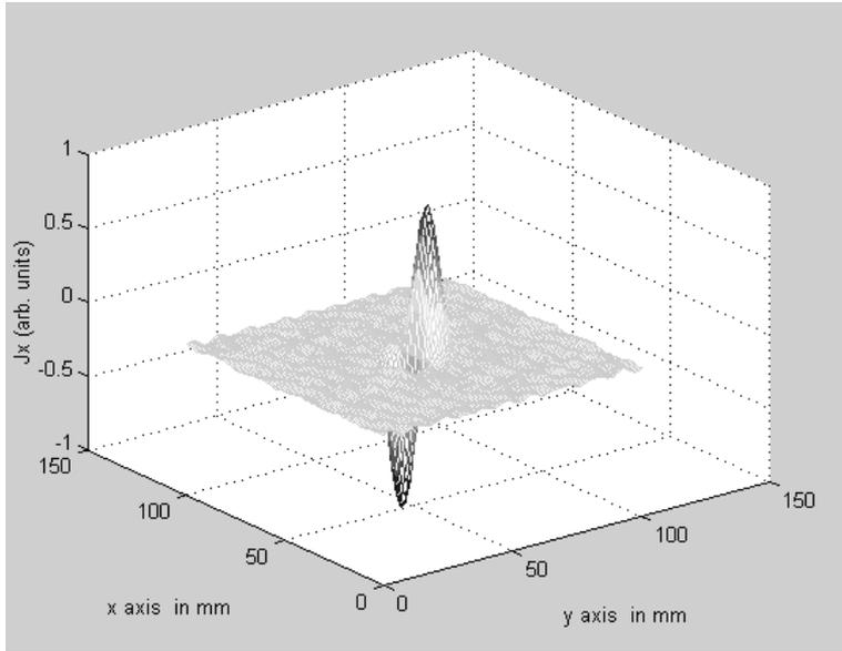
Figure 2. Inverted current density image  $J_x^i(x, y)$ .
