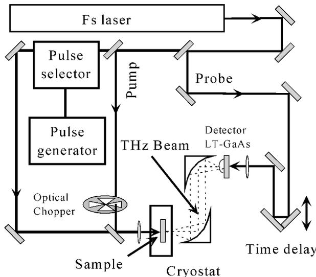
**Figure 2.** Experimental set up for optical pulse illumination of the sample with a fs laser and magnetic flux observation by THz radiation imaging.
