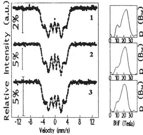
**Figure 2.** Mössbauer spectra of  $\text{Fe}_{40}\text{Ni}_{38}\text{Mo}_4\text{B}_{18}$  metallic glass sample for (1) virgin, (2) irradiated with dose  $5 \times 10^{13}$  atoms/cm<sup>2</sup>, and (3) irradiated with dose  $7.5 \times 10^{13}$  atoms/cm<sup>2</sup>.
