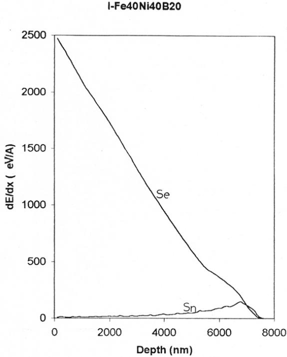
**Figure 1.** Electronic energy loss ( $S_e$ ) and nuclear energy loss ( $S_n$ ) of 90 MeV  $^{127}\text{I}$  beam in  $\text{Fe}_{40}\text{Ni}_{40}\text{B}_{20}$  metallic glass calculated using TRIM.
