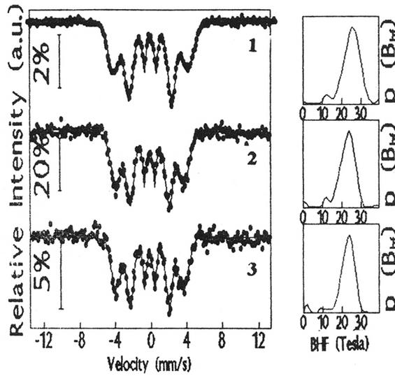
**Figure 3.** Mössbauer spectra of  $\text{Fe}_{40}\text{Ni}_{40}\text{B}_{20}$  metallic glass sample for (1) virgin, (2) irradiated with dose  $5 \times 10^{13}$  atoms/cm<sup>2</sup>, and (3) irradiated with dose  $7.5 \times 10^{13}$  atoms/cm<sup>2</sup>.
