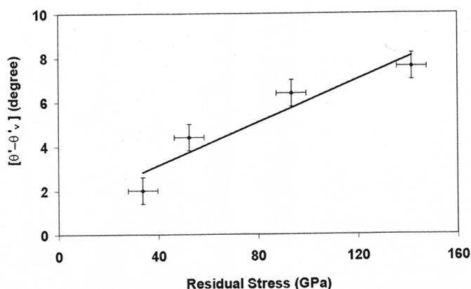
**Figure 4.** Change in average canting angle ( $\theta' - \theta'_v$ ) vs. residual stress giving straight line as a best fit, for the irradiated samples  $\text{Fe}_{40}\text{Ni}_{38}\text{Mo}_4\text{B}_{18}$  and  $\text{Fe}_{40}\text{Ni}_{40}\text{B}_{20}$ .  $\theta'_v$  is average canting angle of the virgin sample.
