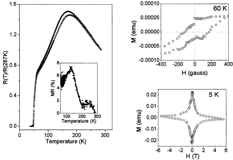
**Figure 2.** (a) The temperature dependence of resistivity for YBCO/LPMO heterostructure (solid and open circles are the data in zero and 1 T magnetic field). The inset shows the variation of magnetoresistance with temperature. (b)  $M-H$  hysteresis loops recorded at 60 K and 5 K.
