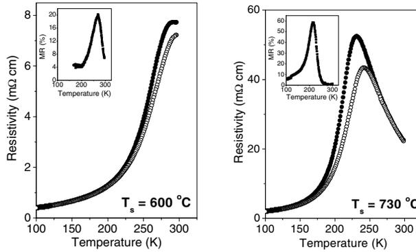
**Figure 1.** The temperature dependence of resistivity for LPMO films grown at different substrate temperatures (solid and open circles are the data in zero and 1 T magnetic field). The inset shows the variation of magnetoresistance with temperature.
