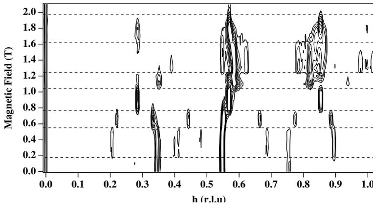
**Figure 2.** Logarithmic contours of neutron diffraction intensities along [h02] as a function of applied field ( $H \parallel [100]$ ) at 1.2 K for  $\text{ErNi}_2\text{B}_2\text{C}$ . This data illustrates the flexibility of the magnetic structure in its response to an applied field and the formation of the vortex state. Note the distinct change at  $H_{C2}$  of 1.3 T.
