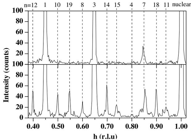
**Figure 1.** Parts of neutron diffraction scans along the  $[h01]$  direction for  $\text{ErNi}_2\text{B}_2\text{C}$  at 2.5 K (upper trace) and 1.7 K (lower trace). The index  $n$  corresponds to harmonic order of the magnetic modulation. The higher temperature data shows the development of a squared moment distribution while below  $T_F$  even harmonics of the modulation become obvious.
