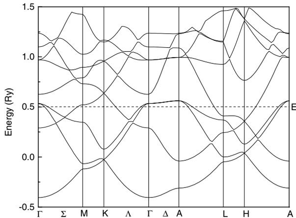
**Figure 1.** Band structure of MgB<sub>2</sub> along different symmetry directions.
