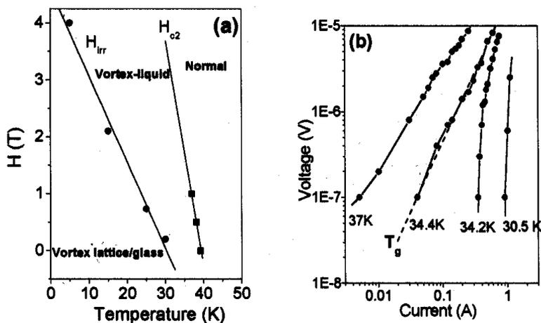
**Figure 1.** (a)  $H$ - $T$  phase diagram showing irreversibility and upper critical field lines. (b) Current-voltage curves obtained at 0.3 T. Dashed line indicates power line behavior at vortex-glass transition temperature ( $T_g$ ).
