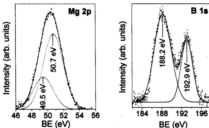
**Figure 2.** Core level Mg 2p and B 1s spectra recorded for the MgB<sub>2</sub> samples exposed to ambient atmosphere for several days.
