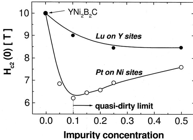
**Figure 4.** Suppression of the upper critical field  $H_{c2}(0)$  of  $YNi_2B_2C$  by Lu impurities on Y sites ( $Y_xLu_{1-x}Ni_2B_2C$  – filled circles) and by Pt impurities on Ni sites ( $Y(Ni_{1-x}Pt_x)_2B_2C$  – open circles). In the latter case, the quasi-dirty limit is reached at  $x = 0.1$ .
