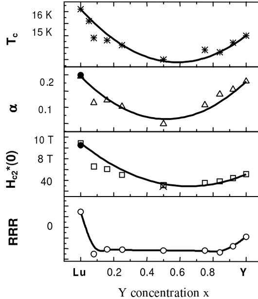
**Figure 2.** Concentration dependence of the superconducting transition temperature  $T_c$ , of the upper critical field parameters  $\alpha$  describing the positive curvature of  $H_{c2}(T)$  and  $H_{c2}^*(0)$  (see eq. (1)) and of the resistivity ratio RRR of polycrystalline  $Y_xLu_{1-x}Ni_2B_2C$ .
