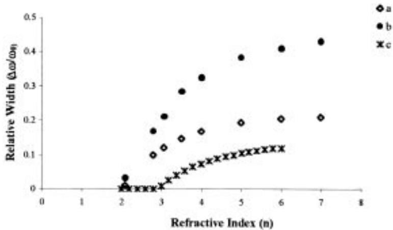
**Figure 2.** Variation of relative width ( $\Delta\omega/\omega_0$ ) with refractive index ( $n$ ) for (a) dielectric sphere, (b) air atom both due to Ho *et al* [2] and for (c) inverted fcc structure.
