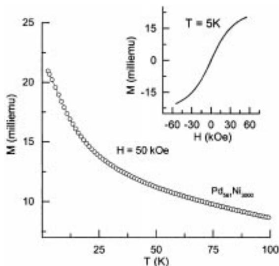
**Figure 2.** Temperature dependence of the magnetization of  $\text{Pd}_{561}\text{Ni}_{3000}$  core-shell nanoparticles capped with octanethiol under an applied field of 50 kOe. The values were corrected for the contribution from the solvent and the glass tube. Inset shows the change in the magnetization (uncorrected) as a function of magnetic field.
