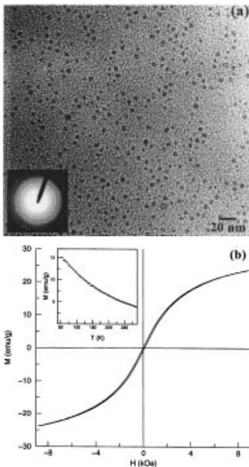
**Figure 6.** (a) TEM micrograph showing  $\text{Fe}_3\text{O}_4$  nanoparticles capped with octylamine. Inset shows the SAED pattern. (b) Hysteresis loop exhibited by the  $\text{Fe}_3\text{O}_4$  nanoparticles. Inset shows the temperature dependence of the paramagnetic moment (under a field of 0.5 kOe).
