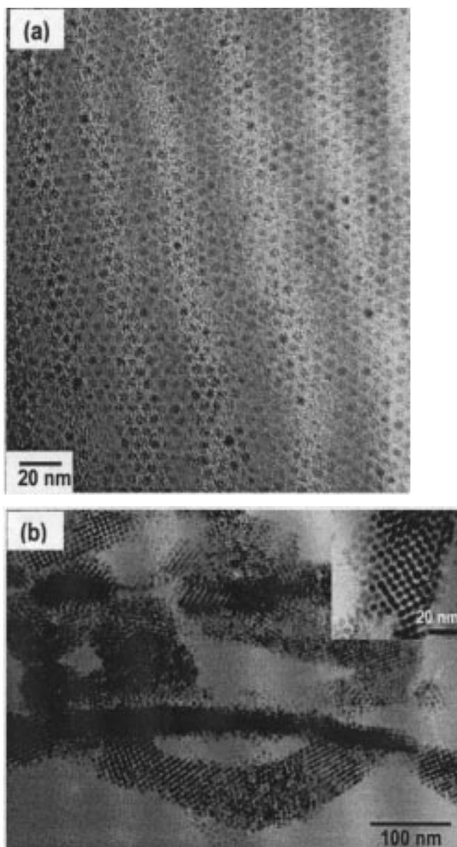
**Figure 1.** TEM micrograph showing arrays of Pd<sub>561</sub>Ni<sub>3000</sub> nanoparticles coated with (a) octylamine and (b) octanethiol.
