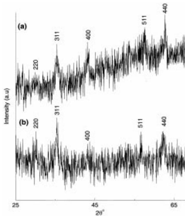
**Figure 4.** X-ray diffraction patterns of (a)  $\gamma$ -Fe<sub>2</sub>O<sub>3</sub> and (b) Fe<sub>3</sub>O<sub>4</sub> nanoparticles.
