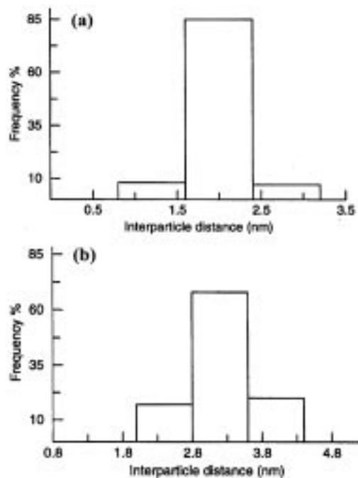
**Figure 9.** Histograms showing the distribution of interparticle distance in the arrays of (a)  $\text{Co}_3\text{O}_4$  nanoparticles capped with octylamine and (b)  $\text{Fe}_3\text{O}_4$  nanoparticles capped with dodecylamine.
