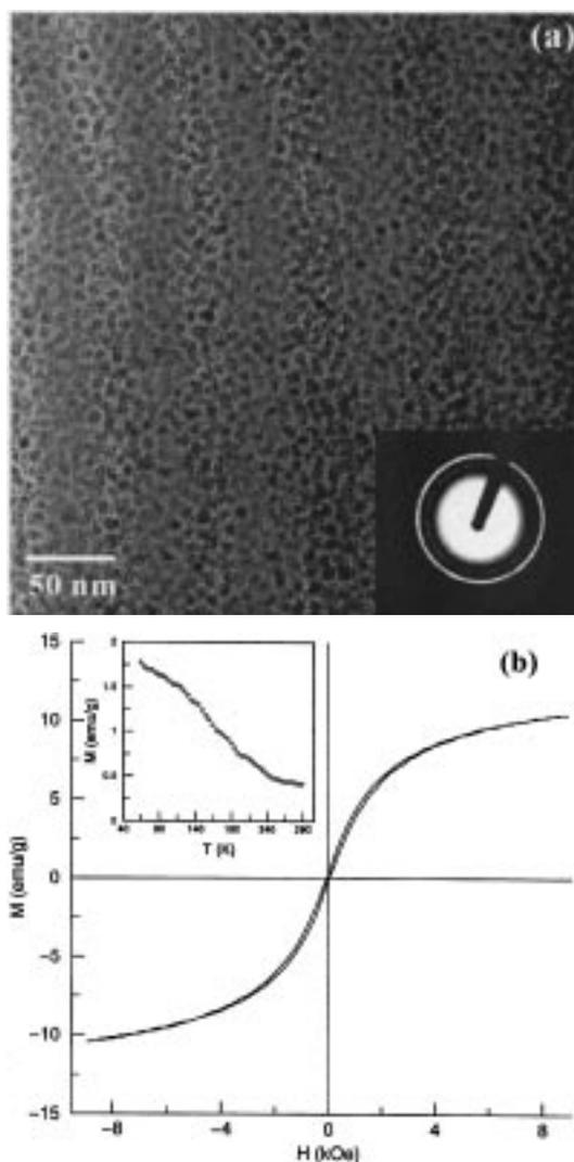
**Figure 5.** (a) TEM micrograph of  $\gamma\text{-Fe}_2\text{O}_3$  nanoparticles capped with octylamine. Inset shows the obtained SAED pattern. (b) Hysteresis loop exhibited by the  $\gamma\text{-Fe}_2\text{O}_3$  nanoparticles. Inset shows the temperature dependence of the paramagnetic moment (under a field of 0.5 kOe).
