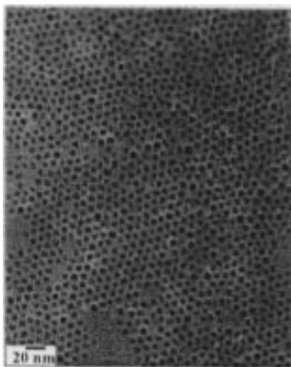
**Figure 3.** TEM micrograph showing arrays of Pd<sub>561</sub>Ni<sub>3000</sub>Pd<sub>1500</sub> nanoparticles coated with octylamine.
