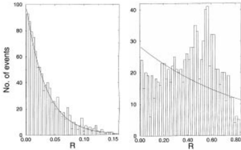
**Figure 1.** The distribution of the reflection coefficient  $R$  for a cavity with one wave guide, supporting one channel: (left) in the presence of strong absorption ( $\langle R \rangle = \alpha = 0.034$ ); (right) for moderate absorption ( $\langle R \rangle = \alpha = 0.410$ ).
