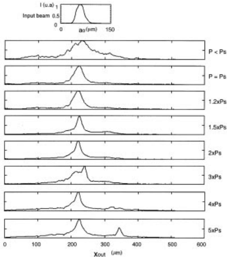
**Figure 5.** Spatial evolution of the output beam with input power  $P$ . Intensity in arbitrary units versus dimension  $x$ . (a): entrance beam, (b): output beam for increasing values of  $P$ .
