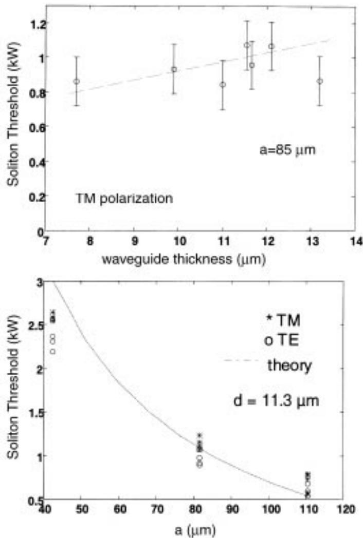
**Figure 7.** Influence of the size parameters  $d$ ,  $a$  on the soliton power  $P_s$ . (a)  $P_s$  versus  $d$  for  $a = 85 \mu\text{m}$  (--- : theoretical curve) (b)  $P_s$  versus  $a$  for  $d = 11.3 \mu\text{m}$  (—: theoretical curve).
