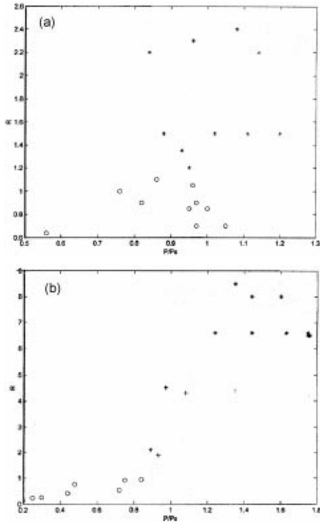
**Figure 17.** Values of  $R = (P_{TE}/T_{TM})$  versus  $P/P_s$ , for  $R_0 = 0.03$ . (a)  $d = 12 \mu\text{m}$ ,  $a = 120 \mu\text{m}$ ; (b)  $d = 12 \mu\text{m}$ ,  $a = 80 \mu\text{m}$ ; o : points without PM and SRWS, \* : points with SRWS, + : points with PM, without SRWS.
