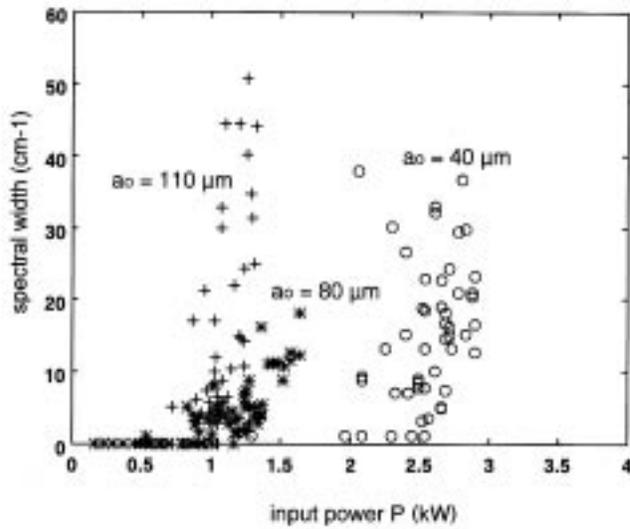
**Figure 10.** Total spectral width versus power  $P$  for 3 cases :  $a = 40 \mu\text{m}$  ( $P_s = 2.4 \text{ kW}$ ),  $a = 80 \mu\text{m}$  ( $P_s = 1.2 \text{ kW}$ ),  $a = 110 \mu\text{m}$  ( $P_s = 0.9 \text{ kW}$ ).
