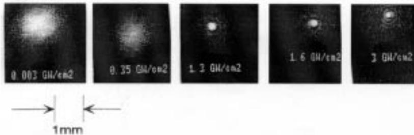
**Figure 2.** Laser beam transverse section at the output of a CS<sub>2</sub> cell (length 0.5 cm) – excitation provided by a mode-locked Nd:YAG laser (duration 30 ps). Intensity ranging from 3 MW/cm<sup>2</sup> to 3 GW/cm<sup>2</sup>.
