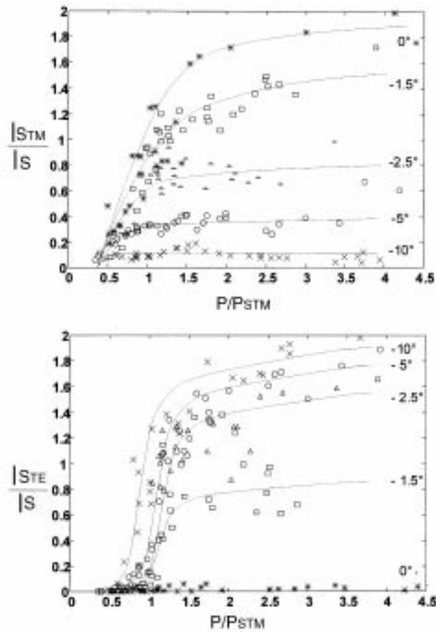
**Figure 12.** Intensity measurements  $I_{TE}$  and  $I_{TM}$  of the two output polarization components measured in the center of the beam ( $x = y = 0$ ) as a function of input power  $P$  for five values of  $\theta$  in the interval  $0^\circ < \theta < 10^\circ$ .
