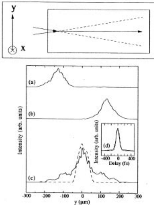
**Figure 5.** The top panel illustrates noncollinear generation of STS and bottom panel presents experimental results. STS produced by one input beam are shown in (a) and (b), and STS produced with both input beams present are shown in (c). The inset shows the temporal profiles of the input pulse and the STS generated by noncollinear SHG.
