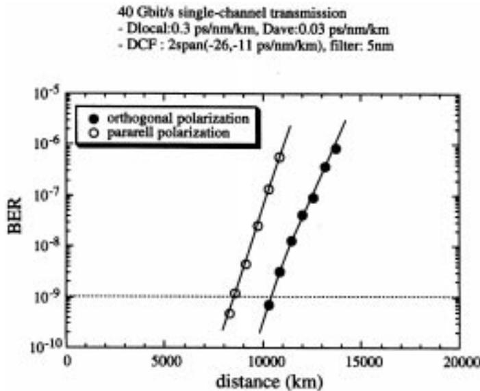
Figure 6. Bit error rate measurement after 10,000 km transmission of the 40 Gb/s soliton signals by Morita *et al* [16]. (°) for parallel polarization and (•) for orthogonal polarization between adjacent pulses.
