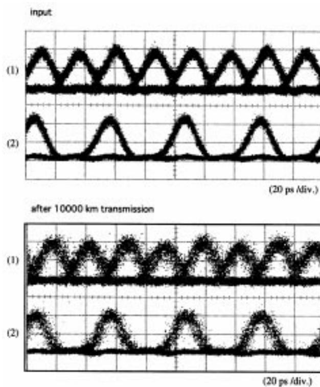
**Figure 7.** Measured eye diagram of soliton pulses after 10,000 km of transmission. The picture is taking by overlaying a sequence of arrived pulses in the bit frame. The opening of the eye indicates error free transmission [16].
