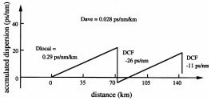
Figure 5. Dispersion map for the 40 Gb/s transmission [16].
