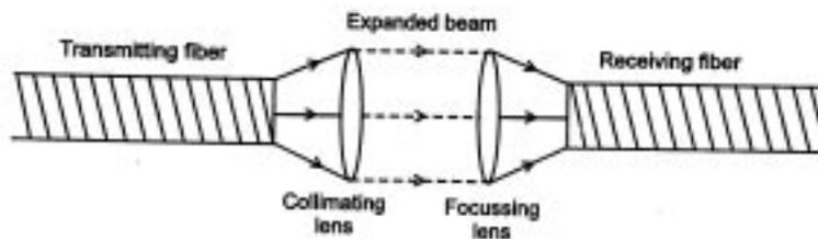
Figure 8. Expanded beam connector.
