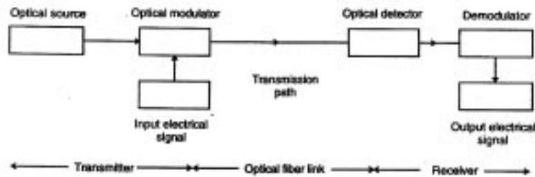
**Figure 2.** Basic analog optical fiber communication system.
