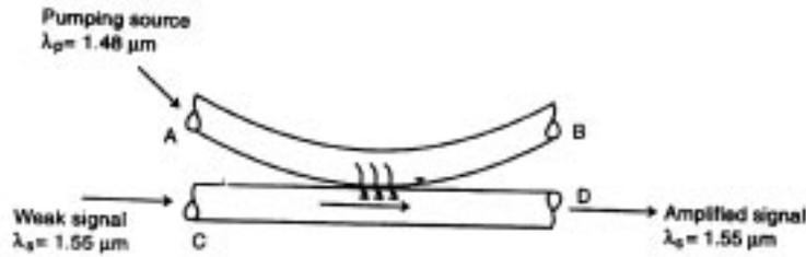
**Figure 4.** Optical fiber laser amplifier.
