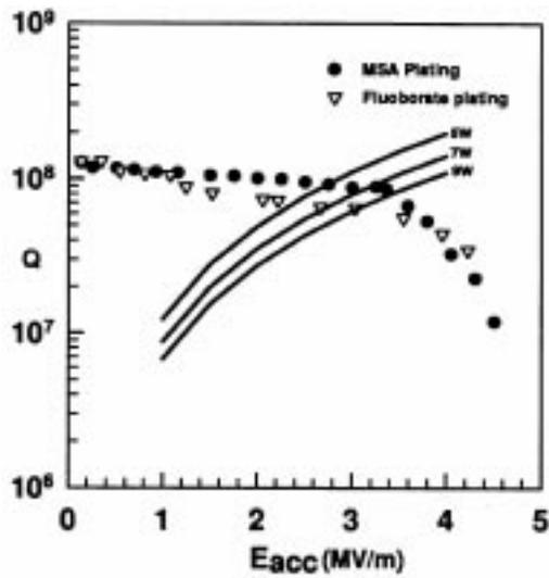
**Figure 3.** Quality factor vs average accelerating field in Seattle resonator for fluoborate and MSA plating.
