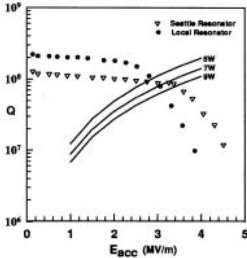
**Figure 4.** Comparison of Seattle resonator and local resonator for fluoborate and MSA plating.
