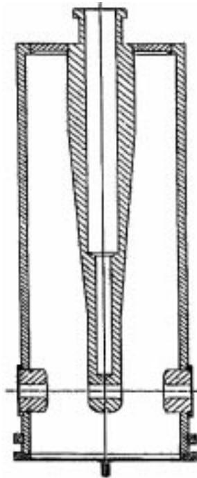
**Figure 2.** QWR schematic.
