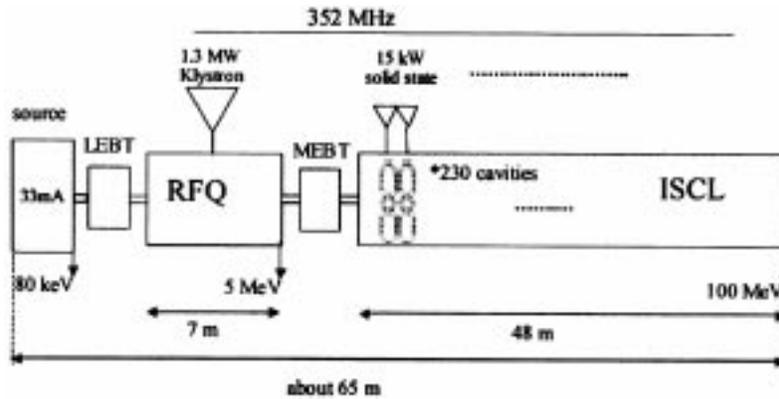
Figure 3. The TRASCO-SPES driver accelerator.
