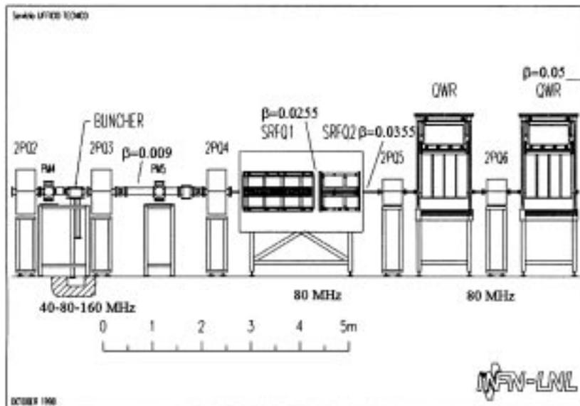
**Figure 11.** PIAVE superconducting injector layout.
