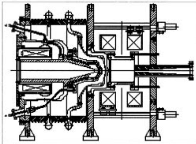
**Figure 4.** The high intensity proton source TRIPS built in Catania (courtesy of INFN-LNS).
