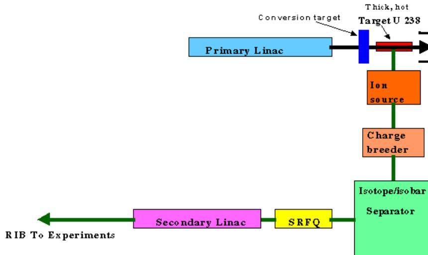
**Figure 1.** Schematic view of the proposed SPES radioactive beam facility.
