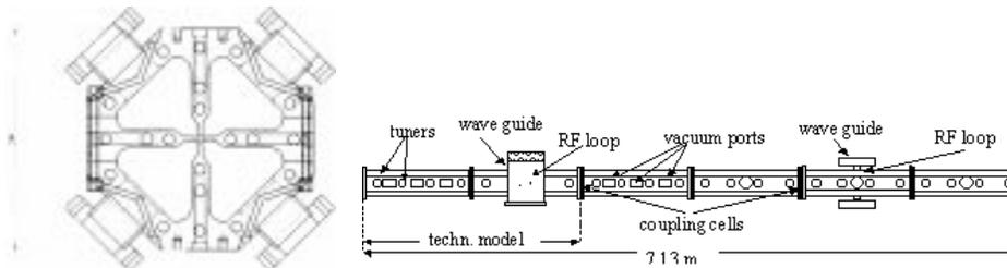
**Figure 5.** Cross section and schematic layout of the TRASCO RFQ.
