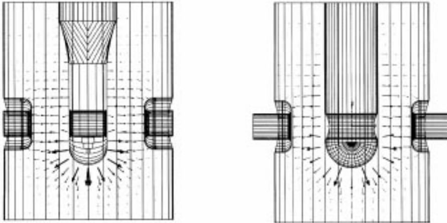
**Figure 10.** The  $\beta = 0.22$  and the  $\beta = 0.25$ , 352 MHz cavities, of the same family of the 80 MHz cavities developed at LNL.
