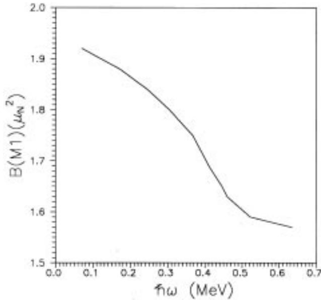
**Figure 6.**  $B(M1)$  vs.  $\hbar\omega$  for the MR band in  $^{105}\text{Sn}$  using the TAC model.
