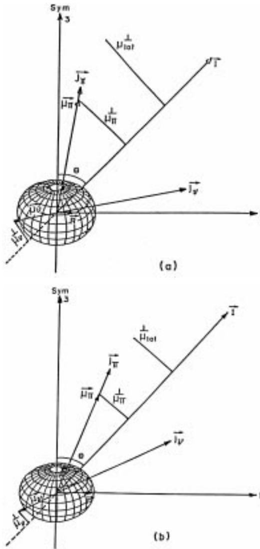
**Figure 2.** Schematic coupling scheme of shears mechanism for a small oblate deformation at (a) small rotational frequency, and (b) larger rotational frequency.
