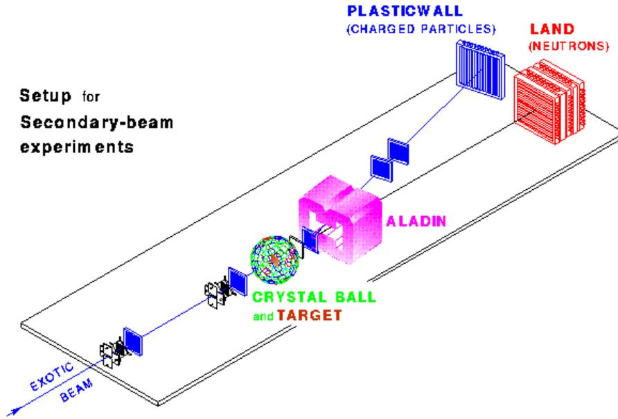
Figure 1. Schematic view of the setup in the experimental area.
