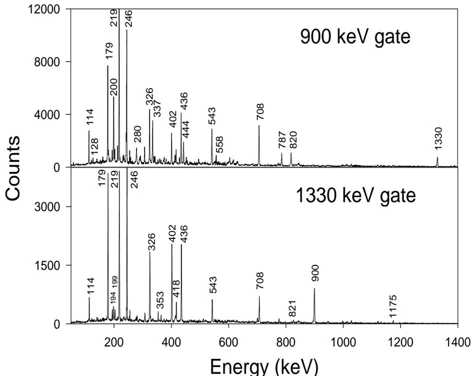
**Figure 1.** Representative  $\gamma$ - $\gamma$  coincidence spectra in the reaction  $^{130}\text{Te}(^{14}\text{N}, 5n)$  at  $E = 75$  MeV, corresponding to selected gates, as indicated.
