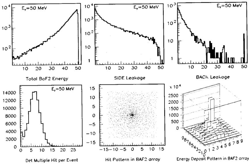
Figure 4. GEANT simulation of 50 MeV  $\gamma$ -rays.
