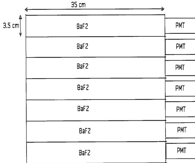
**Figure 1.** Sketch of BaF<sub>2</sub> crystal array.
