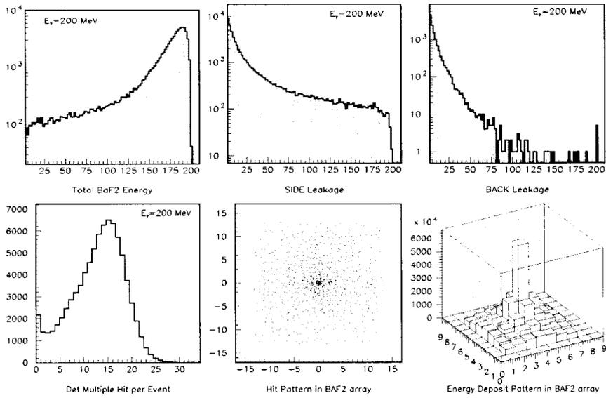
Figure 3. GEANT simulation of 200 MeV  $\gamma$ -rays.
