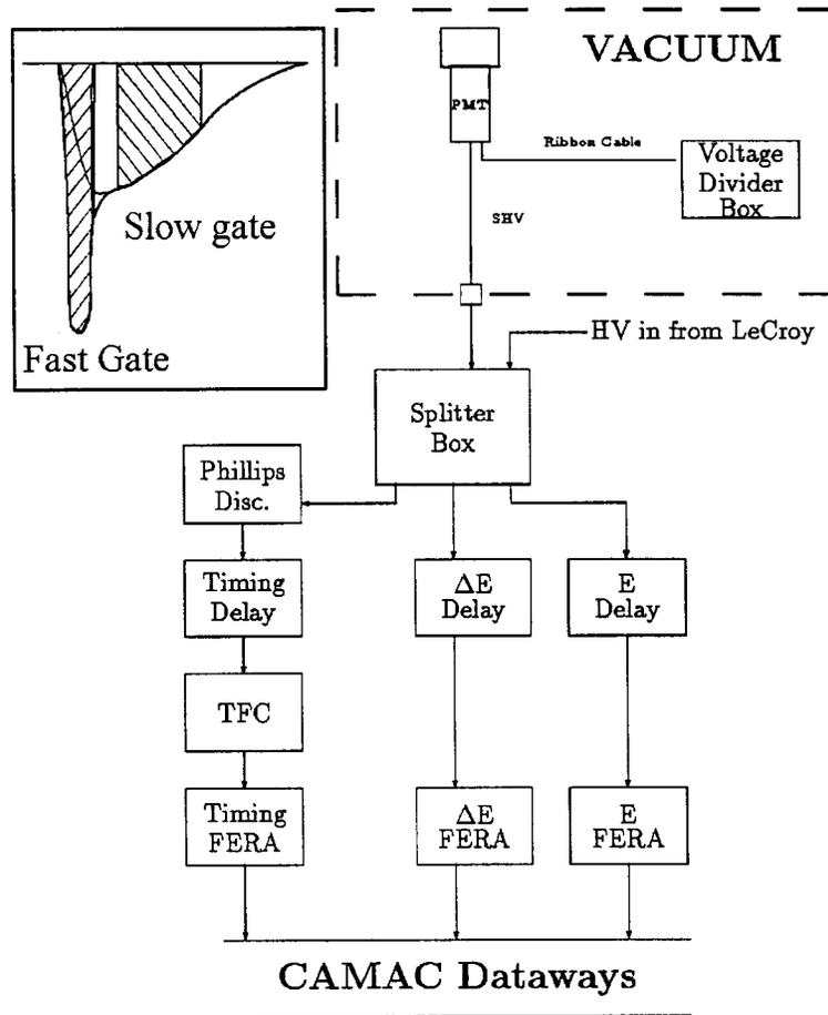
Figure 1. Phoswich detector electronics for MSU  $4\pi$  array.
