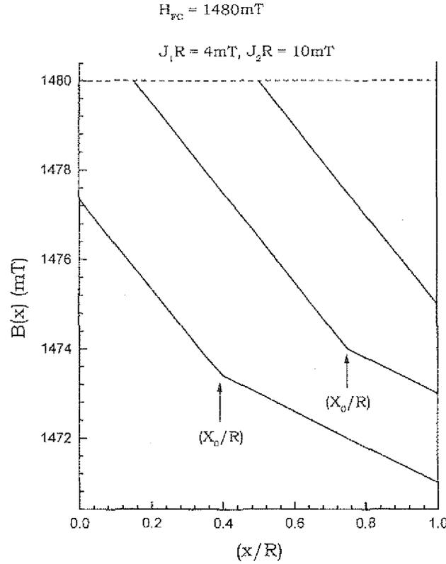
**Figure 3.** The sample is field-cooled in 1480 mTesla, when  $B(x)$  is constant as shown by the dashed line, and vortex matter is in the metastable phase 2.  $B(x)$  are shown as the applied field is lowered isothermally to 1475, 1473, and 1471 mTesla. In the last two fields the vortex matter has transformed to the stable phase 1 at  $x > x_0$ , where  $x_0$  is indicated by an arrow.
