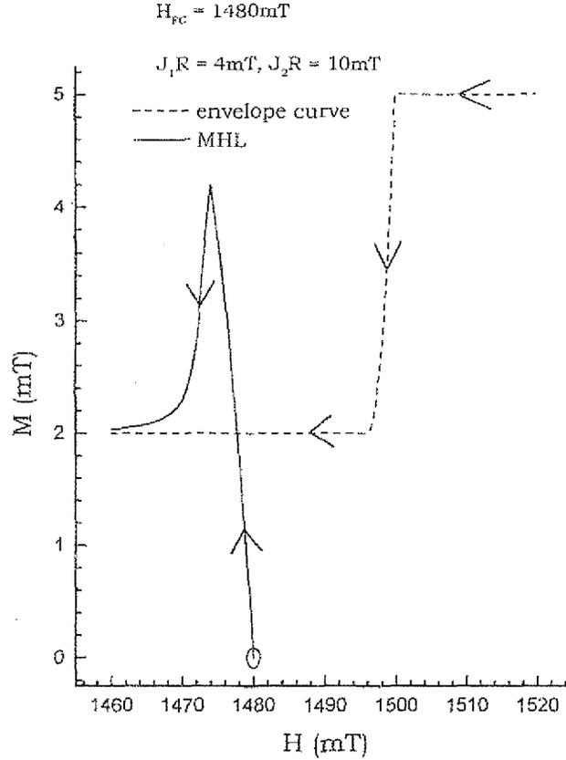
**Figure 4.** MHL obtained after field-cooling at 1480 mTesla is shown by the solid line. It overshoots the envelope curve, and merges with it slowly from above. The circle indicates the starting point of the MHL, with  $M = 0$  corresponding to the constant  $B(x)$ .
