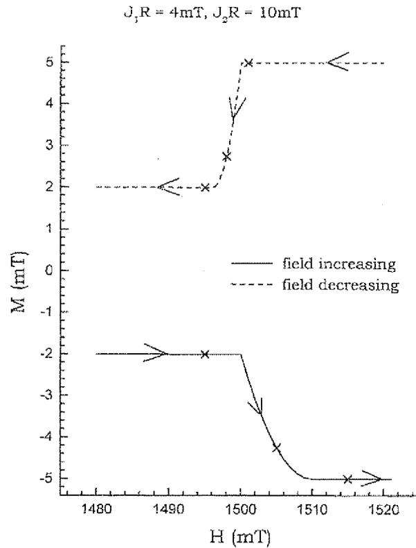
**Figure 1.** Field-increasing and field-decreasing envelope  $M$ - $H$  curves are shown, following the model of eq. (1), with  $B_1 = 1500$  mTesla. The crosses indicate applied field values at which  $B(x)$  profiles are shown in figure 2.
