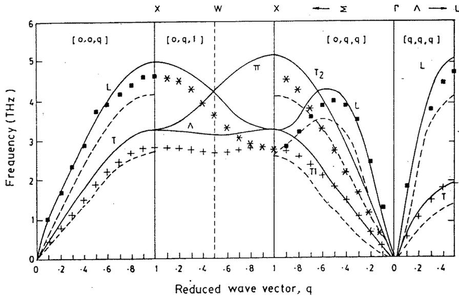
**Figure 6.** Phonon dispersion curves for gold. Continuous lines show results of third order (present work) and dotted lines show results due to Moriarty [31]. Experimental points are due to Lynn *et al* [38].
