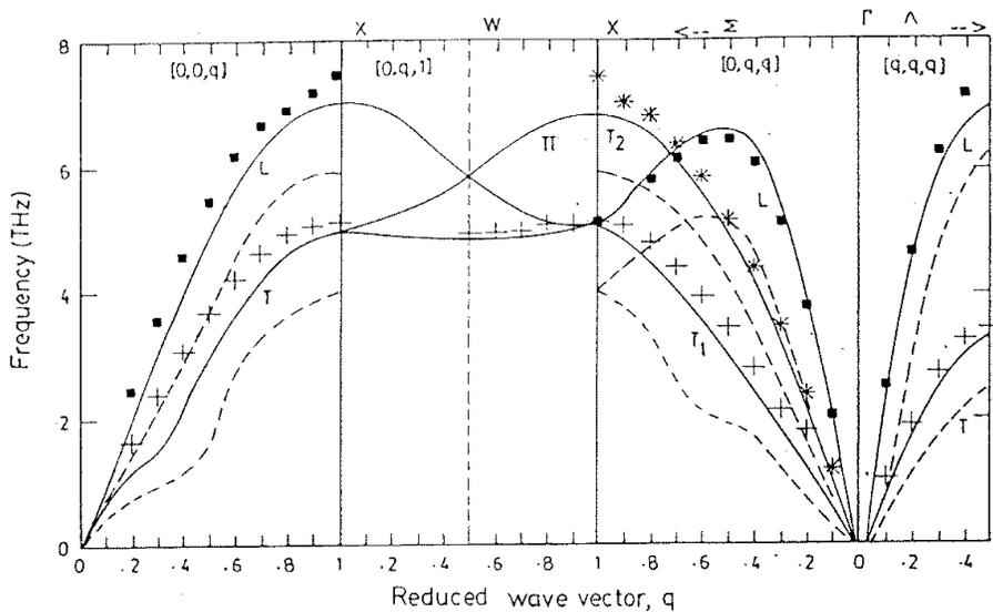
**Figure 4.** Phonon dispersion curves for copper. Continuous lines show results of third order (present work) and dotted lines show results due to Moriarty [31]. Experimental points are due to Nilsson and Rolandsson [36].
