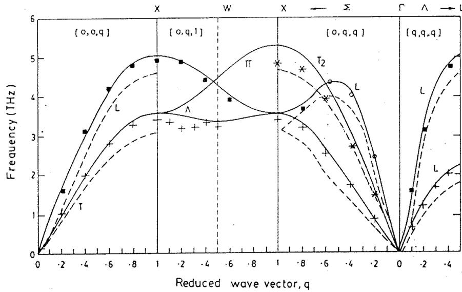
**Figure 5.** Phonon dispersion curves for silver. Continuous lines show results of third order (present work) and dotted lines show results due to Moriarty [31]. Experimental points are due to Kamitakahara and Brockhouse [37].
