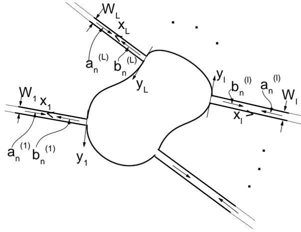
**Figure 2.** The 2D cavity referred to in the text. The cavity is connected to the outside via  $L$  waveguides. The arrows inside the waveguides indicate incoming or outgoing waves. In waveguide  $l$  there can be  $N_l$  such incoming or outgoing waves: this is indicated in the figure by the amplitudes  $a_n^{(l)}$ ,  $b_n^{(l)}$ , respectively, where  $n = 1, \dots, N_l$ .
