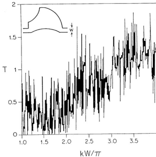
**Figure 3.** Total transmission coefficient of eq. (2) as a function of incident momentum, obtained by solving numerically the Schrödinger equation for the system indicated in the upper left corner. (From ref. [24].)
