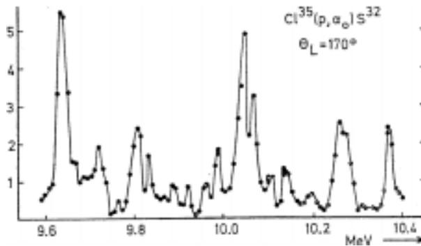
**Figure 1.** The excitation function for the reaction  $^{35}\text{Cl}(p, \alpha_0)^{32}\text{S}$ , in which the residual nucleus  $^{32}\text{S}$  is left in its ground state; the observation is made at  $170^\circ$  in the laboratory. The abscissa indicates the energy of the incident proton. The observed peaks are not individual resonances in the compound nucleus  $^{36}\text{A}$ , but statistical fluctuations produced by the coherent superposition of many resonances. (From ref. [7].)
