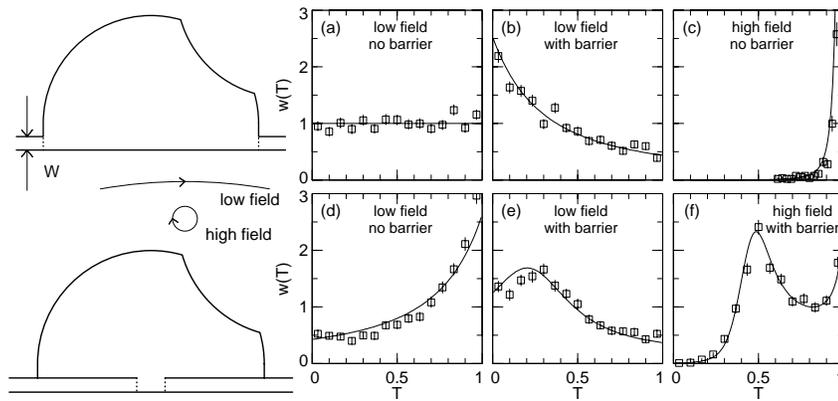
**Figure 6.** The probability density of the total transmission coefficient  $T$  obtained integrating numerically the Schrödinger equation for the billiards shown on the left side of the figure for  $N = 1$ . The results are indicated with squares, that include the statistical error bars. The curves are obtained from Poisson's kernel, eq. (20), with  $\langle S \rangle$  extracted from the numerical data. The agreement is very good. (From ref. [19].)
