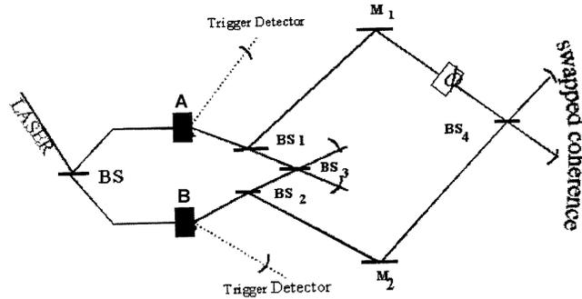
Figure 2. Experimental set up to observe coherence swapping.
