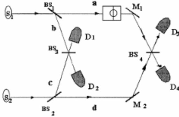
Figure 1. Basic interferometer set-up to observe coherence swapping.
