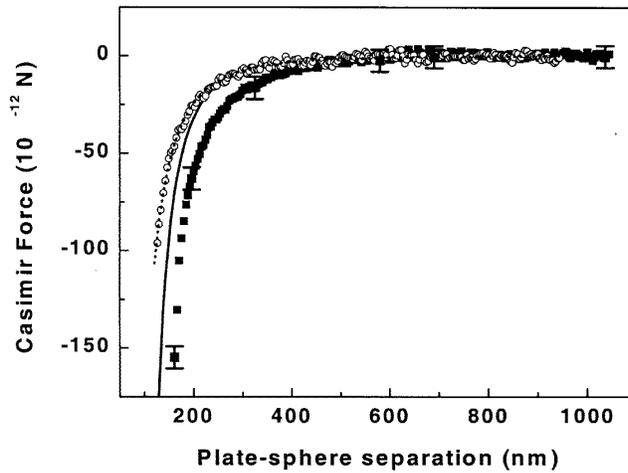
**Figure 2.** Open circles are the measured Casimir force between a flat plate and sphere. Solid squares are the Casimir force between corrugated surface and the same sphere. The solid line is the corresponding theoretical Casimir force using eq. (6) for latter configuration. Dashed line is the theoretical Casimir force obtained by setting  $A = 0$  in eq. (6) for the former configuration.
