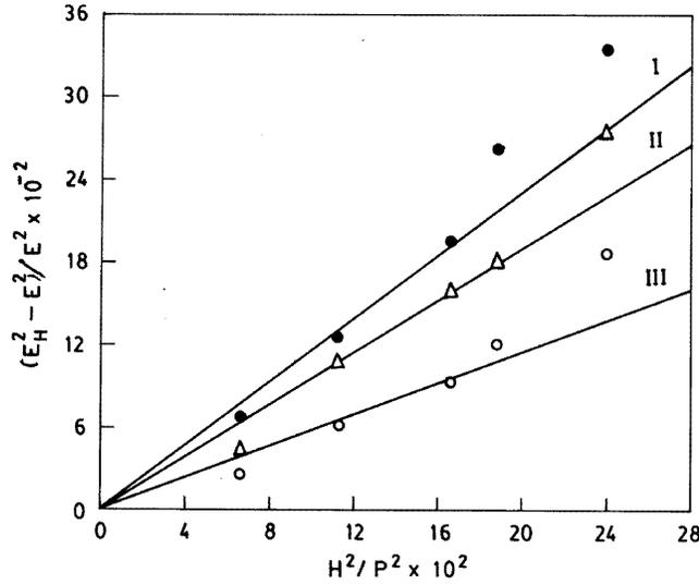
Figure 6. Variation of  $(E_H^2 - E^2)/E^2$  against  $H^2/P^2$ . Initial tube current (I)  $100 \mu\text{A}$ , (II)  $120 \mu\text{A}$ , (III)  $150 \mu\text{A}$ .
