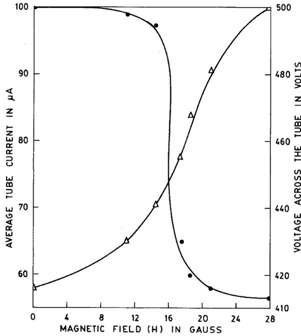
**Figure 3.** Variation of average tube current and axial voltage across the tube. Initial tube current 100 μA.
