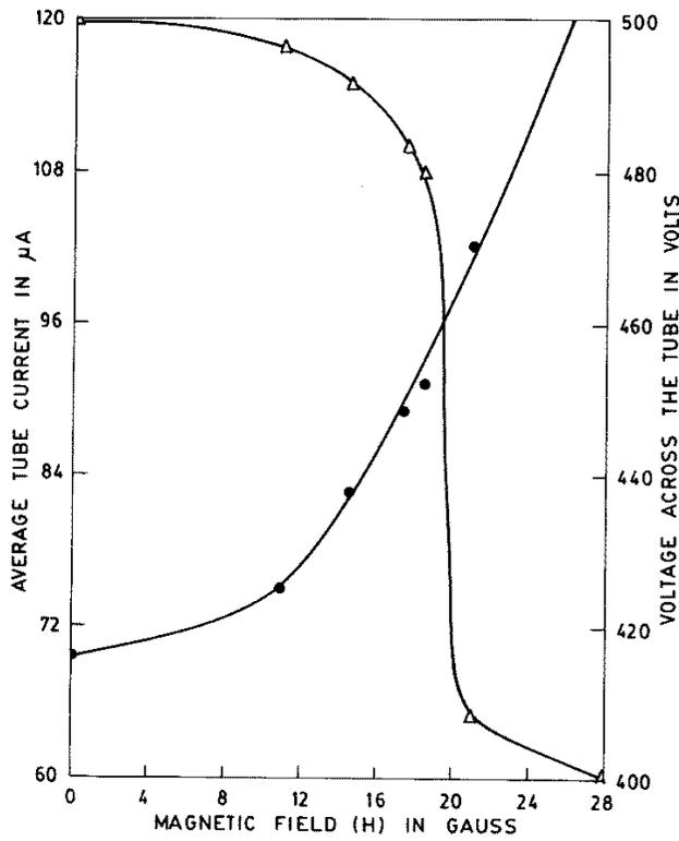
Figure 4. Variation of average tube current and axial voltage across the tube. Initial tube current 120 μA.
