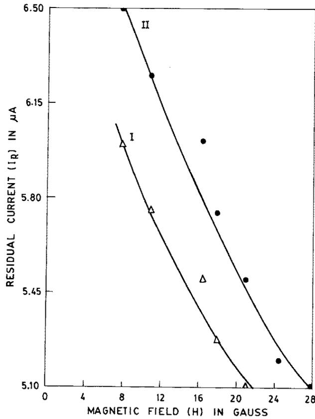
**Figure 5.** Variation of residual current with magnetic fields. Initial tube current (I) 90  $\mu\text{A}$ , (II) 150  $\mu\text{A}$ .
