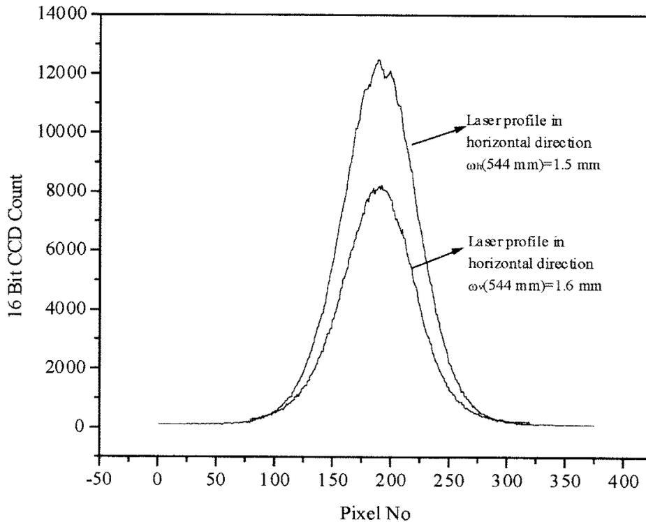
**Figure 3.** Recorded profile of the laser beam at 170 mW pump power. Size of the beam was estimated by fitting zeroth order Hermite–Gaussian intensity profile.
