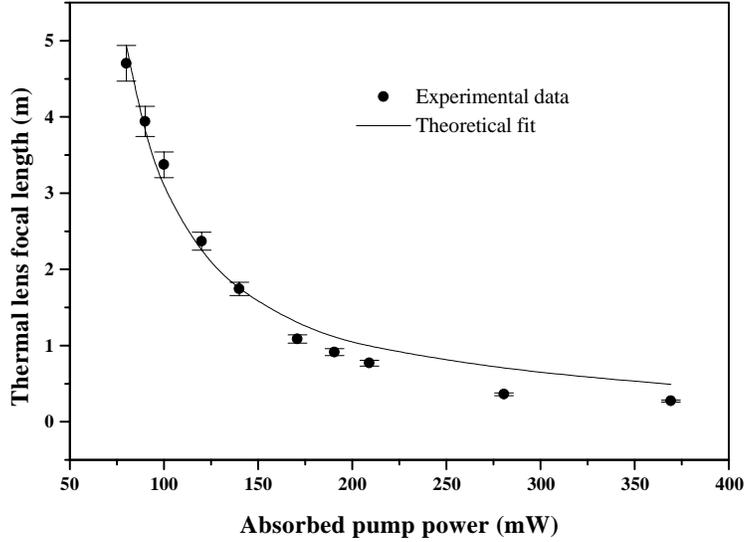
**Figure 4.** Variation of thermal lens focal length with pump power in end-pumped Nd:YVO<sub>4</sub> laser in plane–plane configuration. Focal lengths are estimated by computing mode area at the waist. Dotted curve is the theoretical fit of the function depicted in eq. (11).
