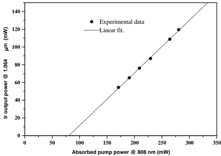
**Figure 2.** Slope efficiency curve for 3 atm% doped 0.5 mm thick Nd:YVO<sub>4</sub> crystal in plane–plane resonator configuration. Nd:YVO<sub>4</sub> laser shows a slope efficiency of 59% and absorbed pump power at threshold is 80 mW.
