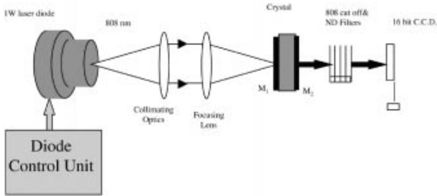
**Figure 1.** Experimental setup for threshold and focal length of thermal lens measurement of diode pumped Nd:YVO<sub>4</sub> microchip laser.
