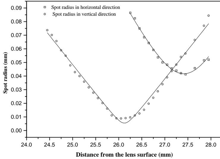
**Figure 5.** Variation of the spot radius of diode laser beam with distance from the secondary principal plane of the focussing lens in horizontal and vertical directions. The continuous line is the theoretical fit of the beam propagation equation in order to find out waist radius, waist location and beam quality factors in the respective directions.
